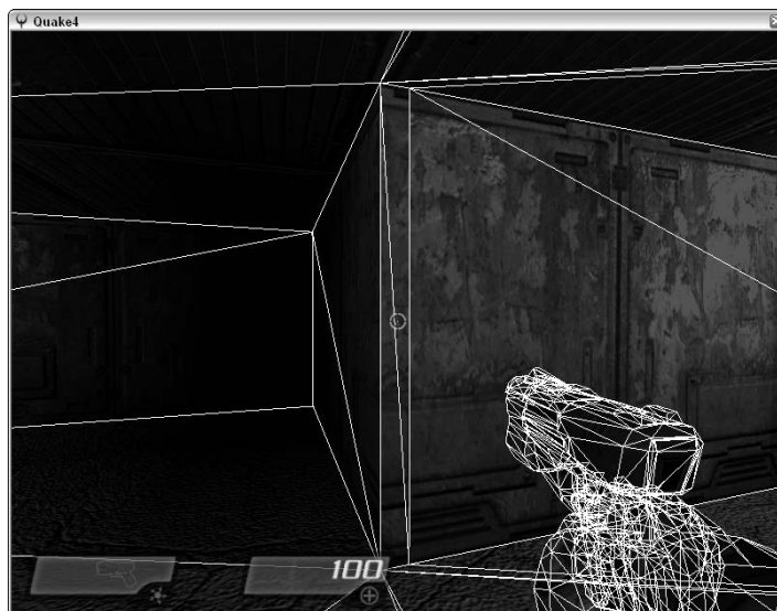
Figure 10-3: Failing to miter corners creates additional geometry.
