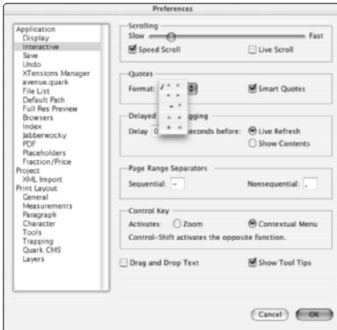
Figure 7-1: Use the Interactive pane of the Preferences dialog box to set up conversion of keyboard quotes.
