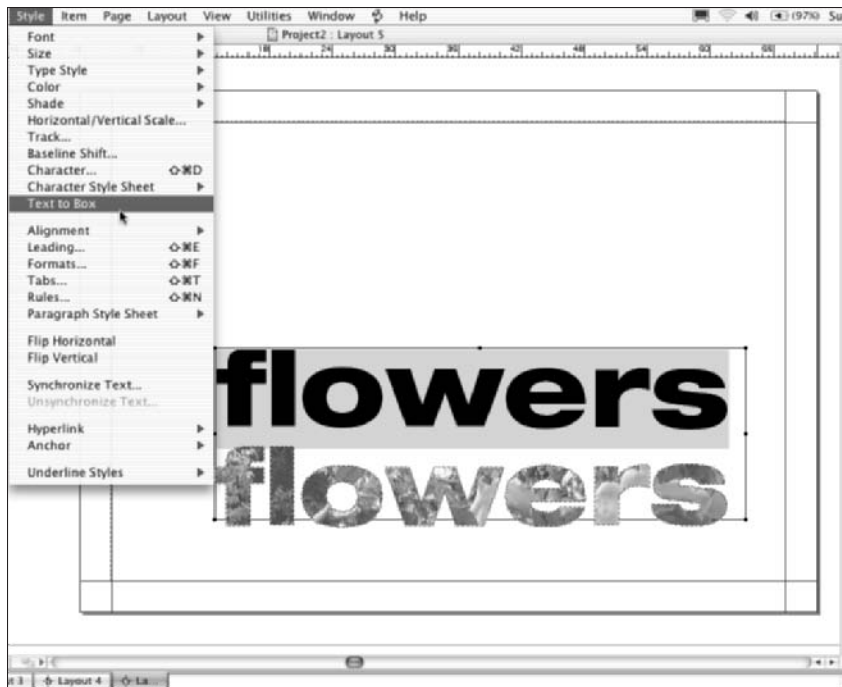
Figure 12-5: Convert text into picture boxes by using the Text to Box command.
