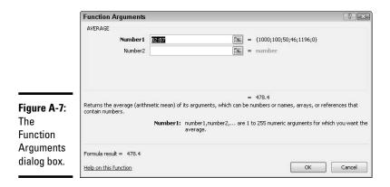
After you supply the needed function arguments, click OK. Excel enters a formula function into the active cell by using the function name and function arguments that you've provided.
