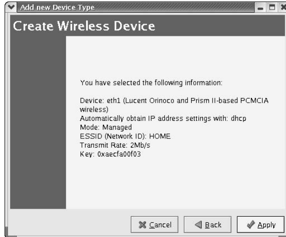
Figure 3-6: Check the information about the wireless connection and click Apply if the information is correct.
