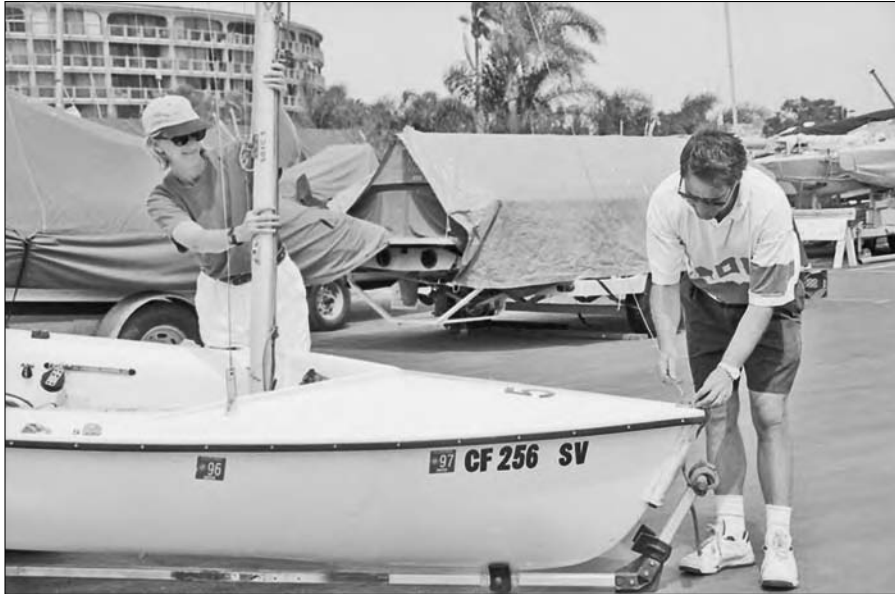
Figure 6-10: One person holds the mast while the second person secures the shrouds and forestay.
