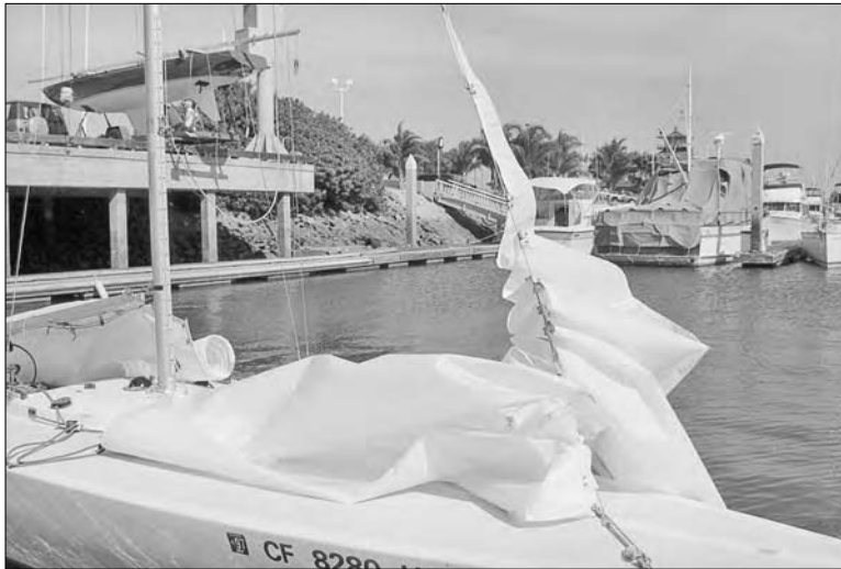
Figure 4-10: This jib is ready to hoist, with the snaps attached to the forestay.
