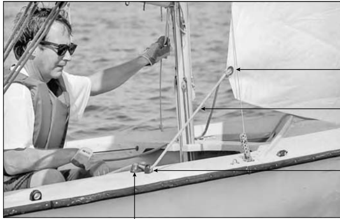
Figure 4-11: Jib sheet system on a 420-class dinghy.
