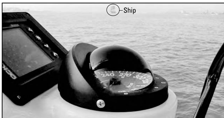
Figure 9-5: Taking a bearing: The ship in the distance bears about 253°.
