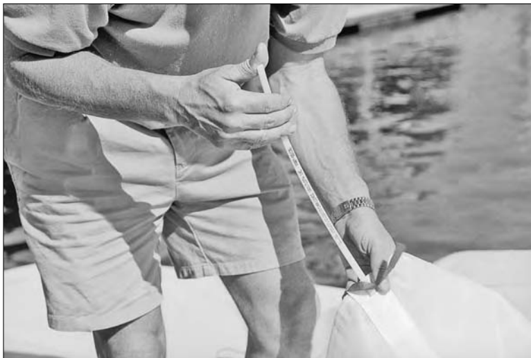
Figure 4-7: Insert battens into the pockets along the sail's leech.
