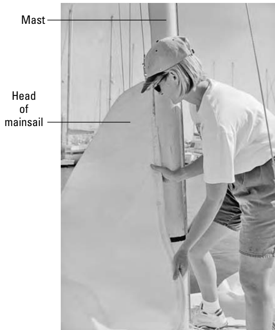
Figure 4-12: Feeding the mainsail luff into the groove in the mast during hoisting.
