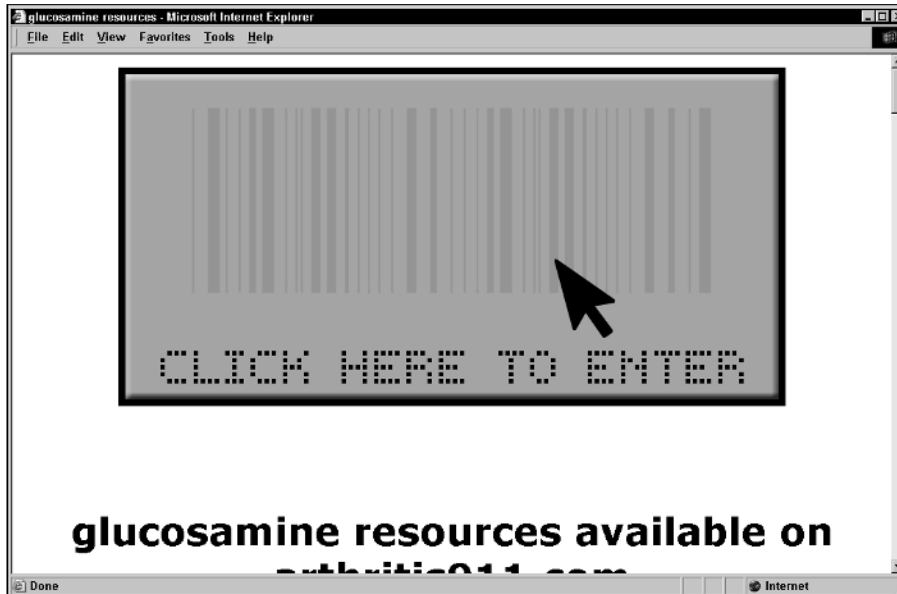
Figure 8-3: The mouse pointer triggers a JavaScript mouseover event on the image, loading another page.
