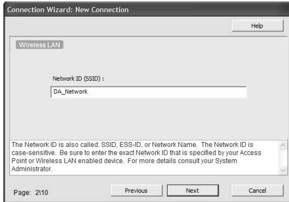
Figure 15-11: Enter the SSID of the wireless network that you want to connect to.
