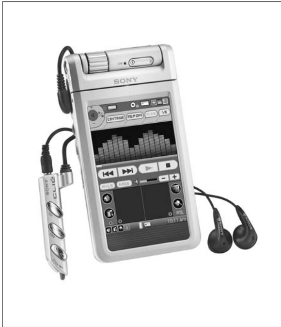
Figure 10-1: Some CLIÉs include not just a headphone jack, but an external audio remote control, as well.
