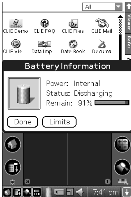
Figure 2-6: The Battery Status meter tells you how much juice is remaining and whether the battery is currently charging.
