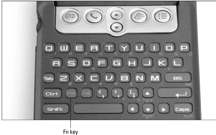
Figure 2-23: Use the Fn key to access numbers and punctu- ation.
