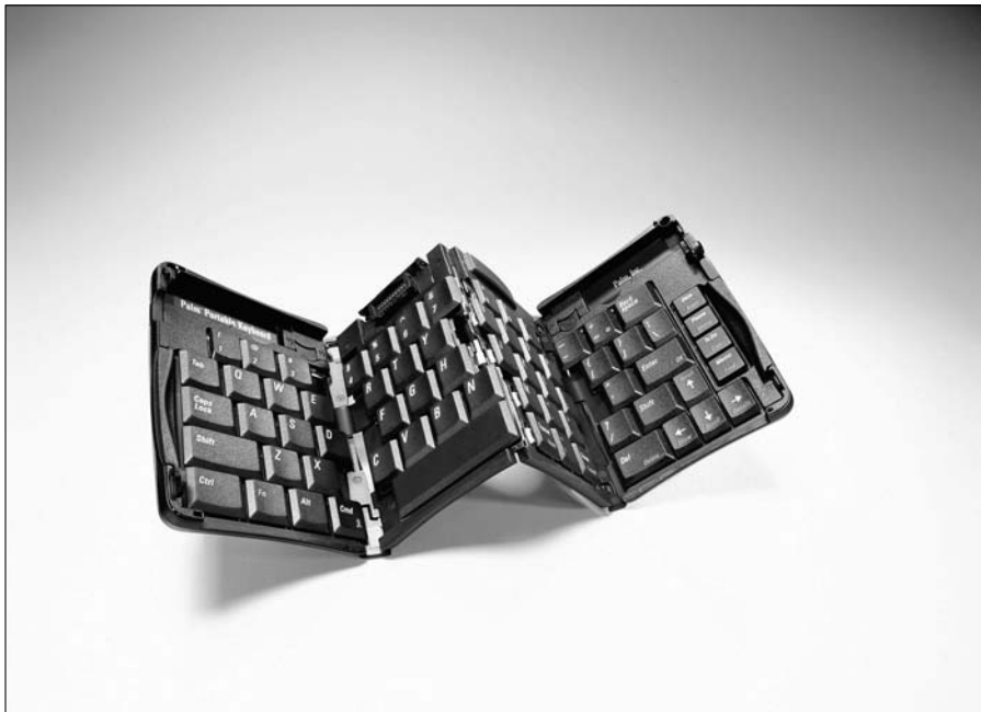
Figure 17-3: The original Stowaway folds into a compact package and unfolds to full laptop keyboard size.
