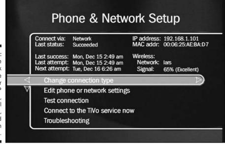
Figure 11-8: TiVo's Phone & Network Setup page lists your network's IP address, signal strength, and connection information.
