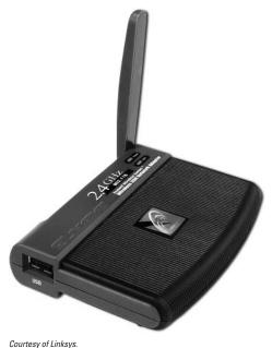
TiVo's adapters are easy to install. Just push the adapter's plug into one of TiVo's USB ports around back. (Leave TiVo turned on.) Keep your wireless adapter's antenna or cable visible; you'll be pushing it around to get a stronger signal, just as early TV owners tweaked the TV's rabbit ears to get a better picture.
