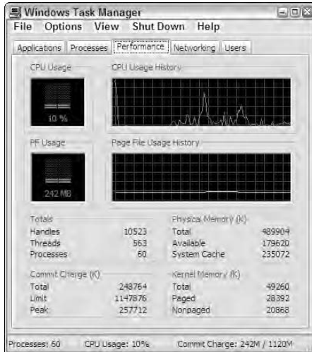
Figure 1-1: A performance report from a laptop under a moderate load. The CPU is lightly loaded and the system has plenty of working room available.
