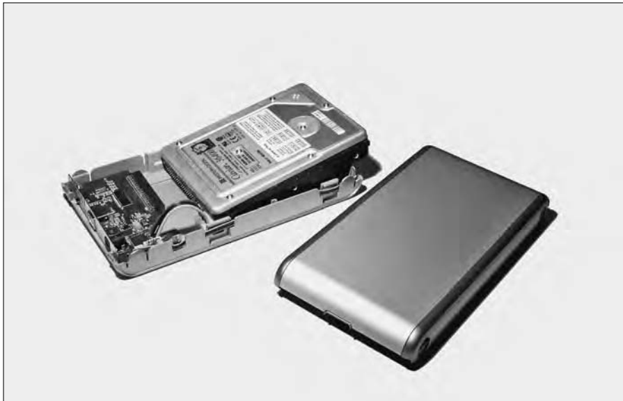
Figure 7-5: An external USB drive kit that recycles a desktop hard drive for use as an attached drive on a laptop.
