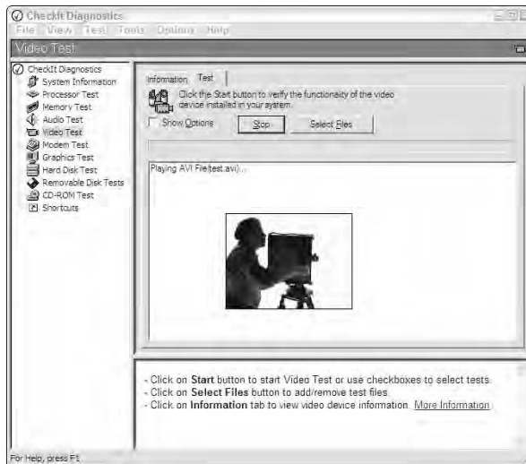
Figure 12-2: Part of the test of a laptop's video card, a component of CheckIt Diagnostics. In this section the utility is testing an AVI video file.
