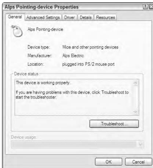
Figure 11-4: The General tab for the pointing device reports that it appears to be working properly. Although this is an internally connected touchpad, the system considers it a piece of hardware that is plugged in to a PS/2 mouse port.
