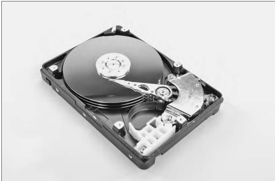
Figure 7-1: Inside a modern hard drive, its internal platters exposed.
