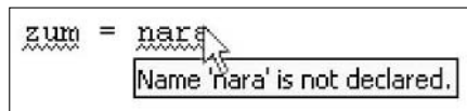
Figure 10-1: A brief error message appears when you pause your pointer on top of an error in the code.
