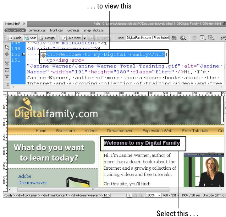
Figure 4-1: Use the Split view option in Dreamweaver to display the page design and the code behind the page.
