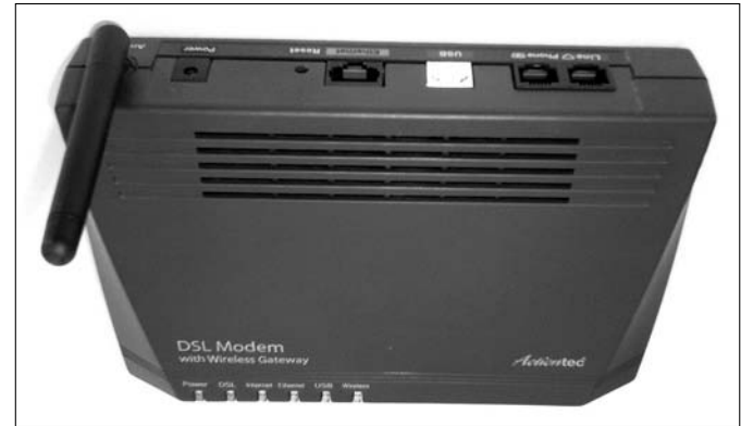
Figure 23-1: This WAP is also a router and a DSL modem.
