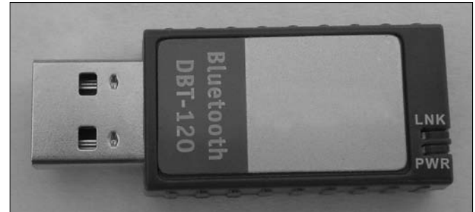
Figure 14-1: This Bluetooth adapter plugs into a USB port.
