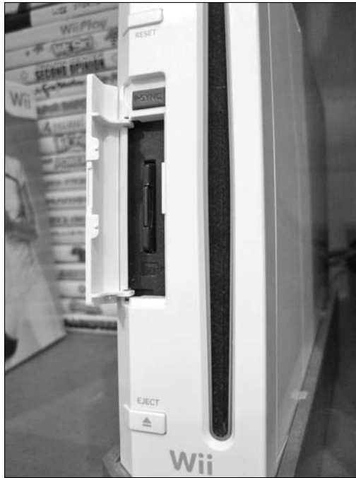
Figure 1-3: The open SD Card slot cover on the front of the Wii console.
