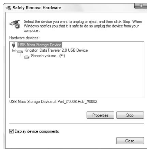
Figure 1-1: Make sure that you tell Vista before you unplug a USB device.
