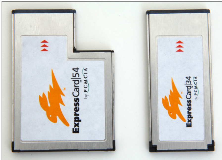
Figure 2-7: PC Card and PC ExpressCard compared.
