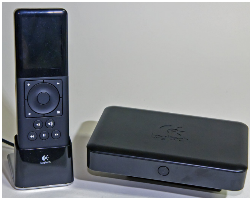
Figure 2-1: The Squeezebox Duet consist of the receiver box and a remote with iPod-like controls and a small LCD screen.
