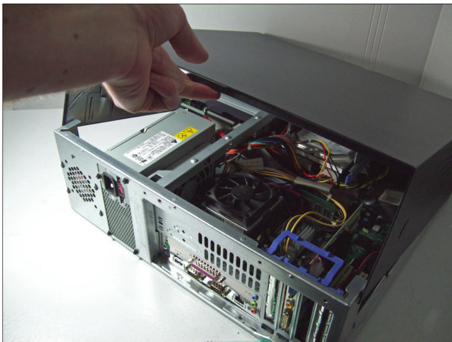
Figure 5-11: Open the case.
