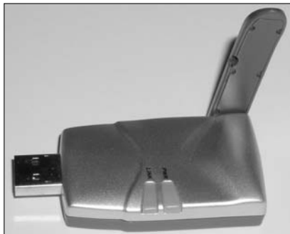
Figure 3-4: Use a USB adapter to add Bluetooth capability to a desktop or laptop PC.
