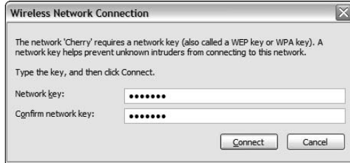
Figure 10-2: Setting up WPA using the Windows XP Wireless Zero Config.
