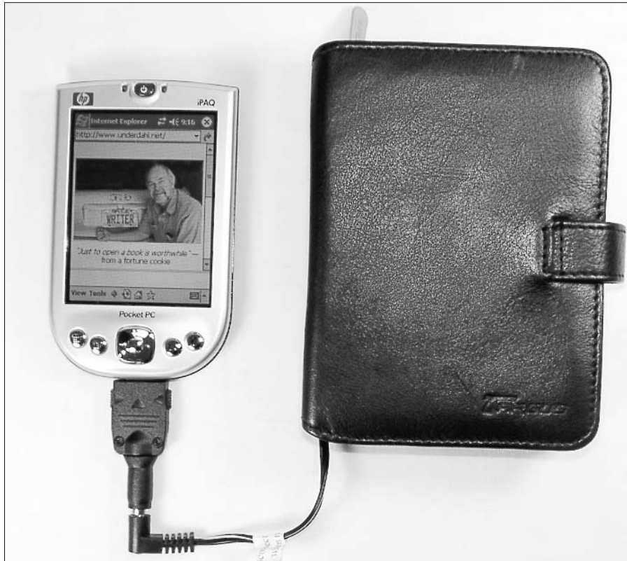
Figure 20-7: The HP iPAQ Auxiliary Battery is a convenient way to double your iPAQ's battery life.
