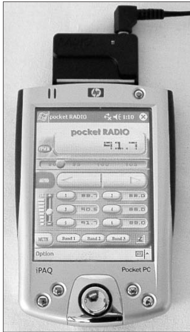
Figure 20-9: The iBIZ pocket- RADIO allows you to listen to your favorite radio sta- tion with your iPAQ.
