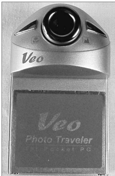
Figure 20-5: The Veo Photo Traveler for Pocket PC is another iPAQ digital camera add-on.
