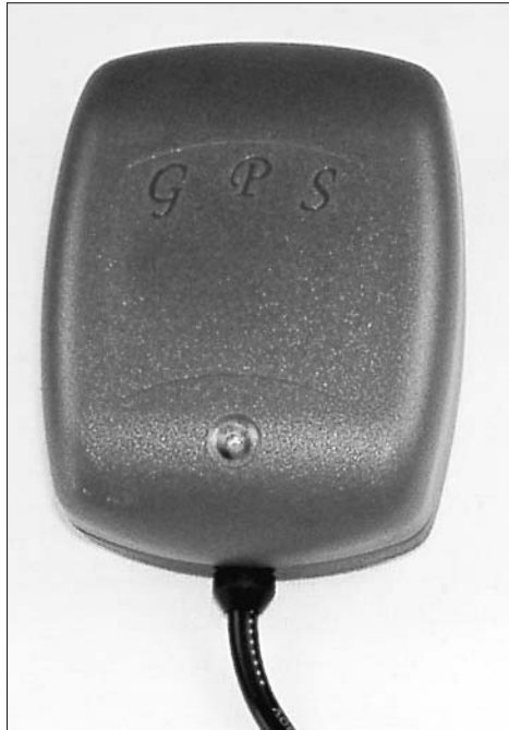
Figure 19-5: The PocketMap Navigator mouse-type GPS receiver plugs into the bottom of your iPAQ.
