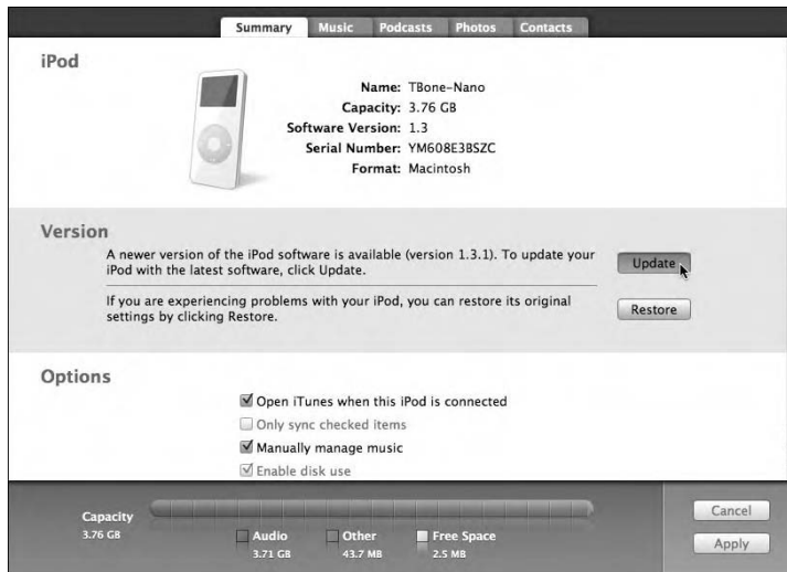
Figure 2-4: iTunes automatically detects new iPod software and lets you update your iPod.
