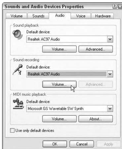
Figure BC2-6: Set audio input and adjust the volume of input for a PC.
