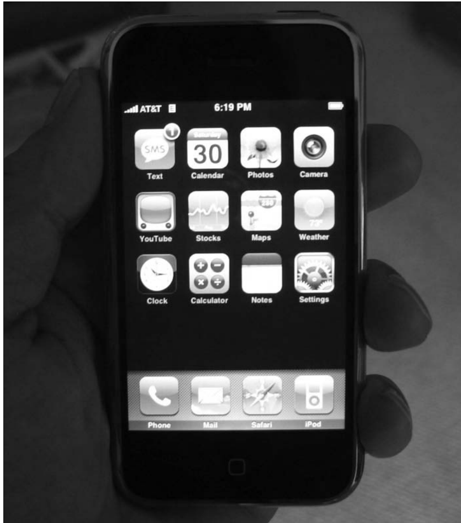
Figure 1-4: The iPhone offers a touch-sensitive display with rich menus and navigational controls.
