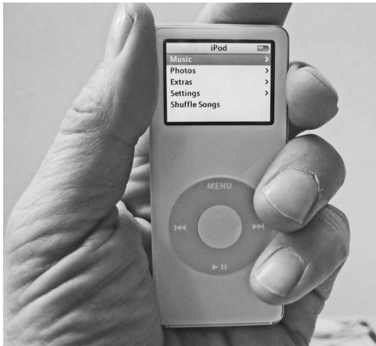
Figure B1-4: iPod nano is the smallest iPod that can display photos as well as menus, calendars, and contacts in color.
