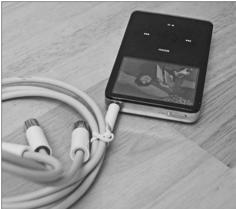
Figure 16-3: The iPod AV Cable provides a yellow video RCA-type connector as well as red and white audio RCA-type connectors.
