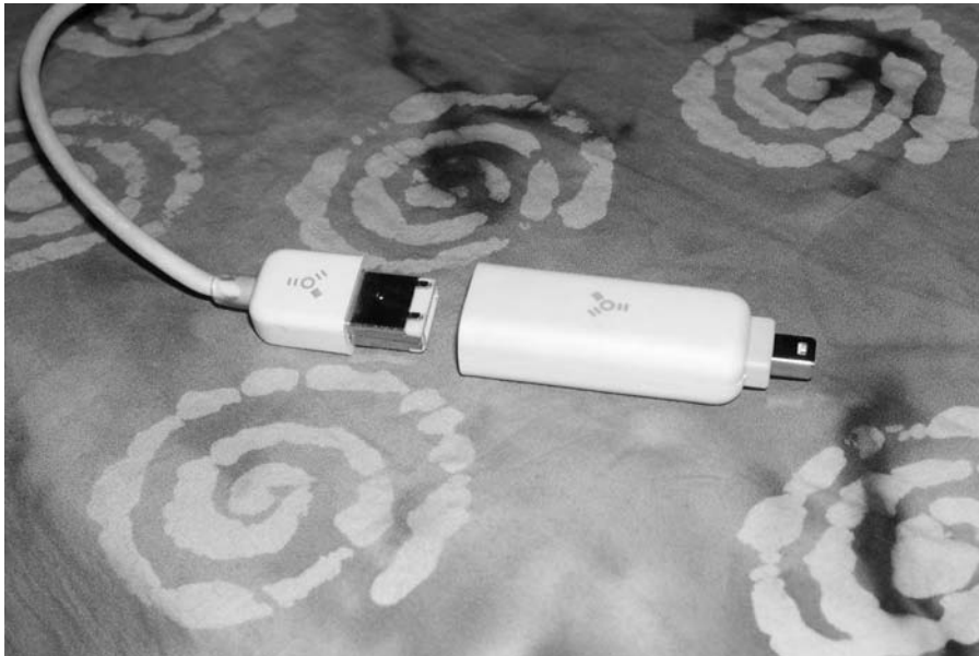
Figure B1-5: The FireWire cable adapter for connecting to a FireWire card that has a four- pin port.
