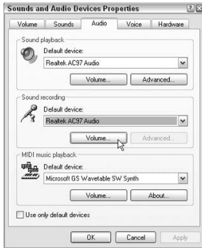
Figure 22-2: Set audio input and adjust the volume of input for a Windows PC.
