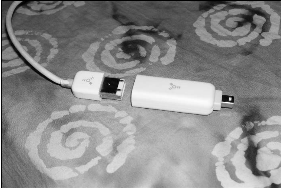
Figure 1-4: The FireWire cable adapter for connecting to a FireWire card that has a four-pin port.
