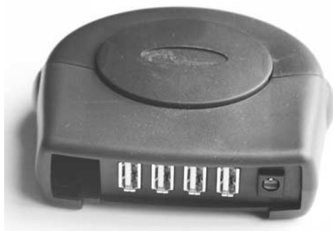
FIGURE 8-5 Belkin's powered USB hub is just one of many options for connecting more USB gadgets to your computer's limited array of USB ports.
