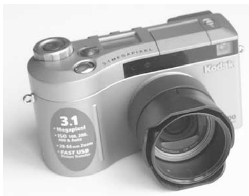
FIGURE 6-2 Lens adapters are a common way to add wide-angle and telephoto lenses to your camera.
