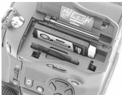
FIGURE 8-2 Most cameras use just one kind of memory, although some newer models—such as the Olympus e10 and e20n—accept both SmartMedia and CompactFlash cards for more flexibility and storage space.
