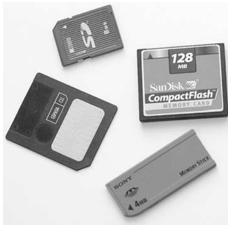
FIGURE 1-5 Four main kinds of memory cards are in use today, and your digital camera is designed to accommodate one of them.
