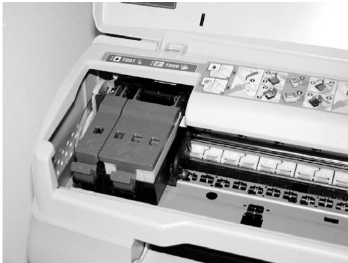
FIGURE 15-2 The print head of an inkjet printer slides back and forth across the page, spraying dots of ink as it goes.
