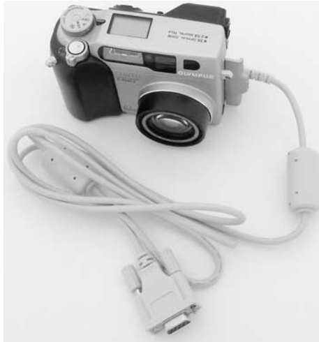
FIGURE 8-3 Transferring images to your PC usually means connecting your camera with a connection cable of some kind. Your camera comes with either a USB or serial cable for this task.
