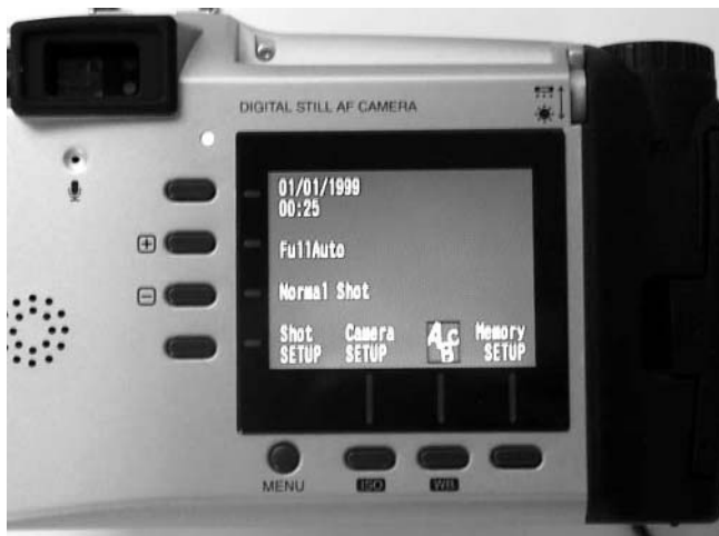
FIGURE 1-7 Digital cameras use a series of menus in the LCD display to operate the more advanced or less frequently used features.
