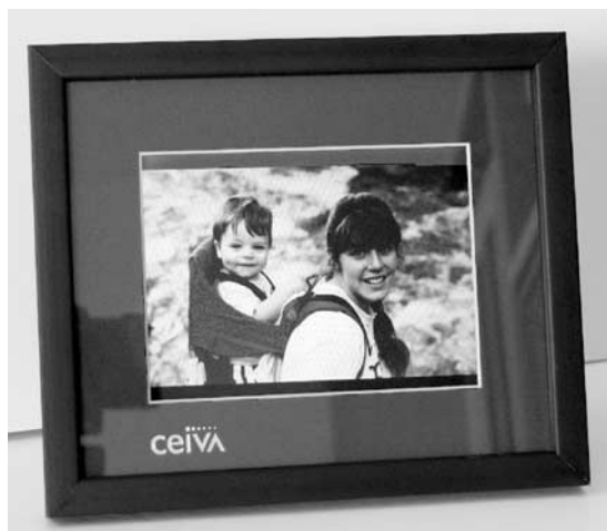
FIGURE 16-10 Digital picture frames put an always-changing slide show of your digital images right on a table top.
