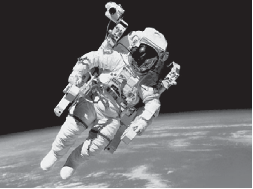
Figure 16.4. Free-floating astronaut in low-earth orbit. The spacesuit contains complete life-support capability for short duration, including protection from radiation, insulation from heat and cold, adequate atmospheric pressure, an O_2 supply, and capacity for CO_2 absorption. Spacesuits are hybrid life-support systems, with many open features that reduce cost and improve reliability. For example, metabolic CO_2 is absorbed and later discarded, the O_2 necessary for the astronaut's activity is stored, not generated, in the suit, heat is dissipated to space by radiation, and wastewater (e.g., sweat and urine) is not recycled. (Source: National Aeronautics and Space Administration.)
