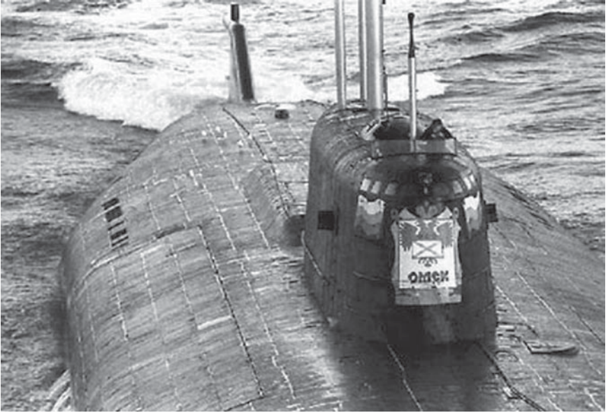
Figure 14.1. Oscar-II Class Russian submarines, one of eleven, the Kursk was lost in the Barents Sea on August 12, 2000, with 118 men aboard. The Kursk 's sister ship, the Omsk , is shown here at sea. Initially, twenty-three men survived a pair of explosions in the forward torpedo room that drove the submarine into the bottom in 456 feet (137 meters) of water. Unfortunately, the survivors could not be rescued.
