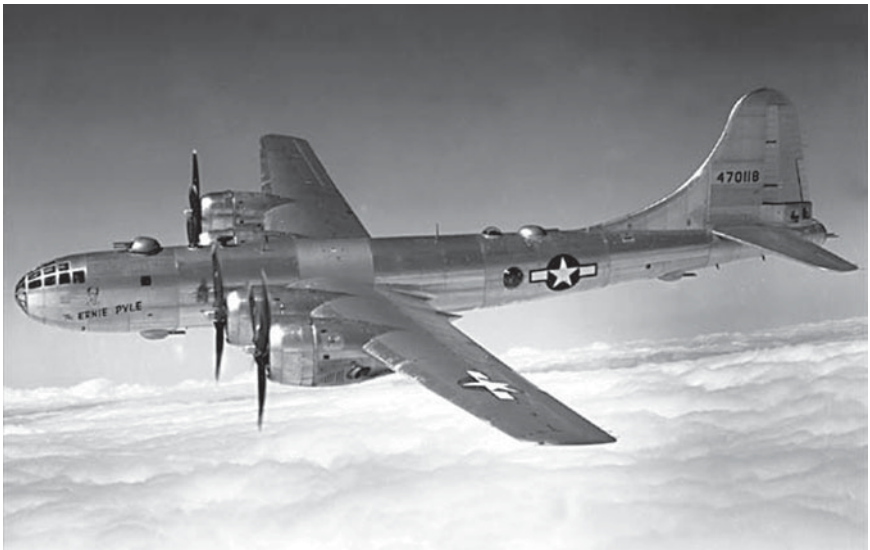
Figure 13.1. The B-29 Superfortress was the first aircraft to fly in combat with a pressurized cabin. The bomber's service ceiling of more than 30,000 feet enabled it to fly into the stratosphere, above antiaircraft fire. During World War II some 2000 of these bombers were employed in the Pacific, and two, Enola Gay and Bock's Car , dropped atomic bombs on Hiroshima and Nagasaki in August 1945. (Copyright The Boeing Company, reproduced with permission.)
