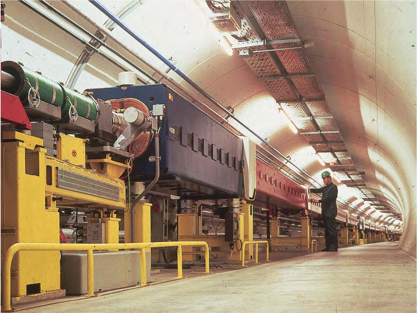
**Fig. 6.36** The tunnel of the Super Proton Synchrotron (the SPS), in the weeks before the machine accelerated its first protons in 1976. The SPS became the world's first proton-antiproton collider in 1981, and remains in use to this day as part of CERN's network of accelerators.
