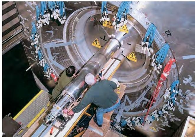
**Fig. 8.35** (BOTTOM RIGHT) Technicians install the new 'silicon microvertex detector' at the centre of the ZEUS experiment at DESY. The detector measures charged particle tracks to 0.01 mm and allows the experiment to pinpoint the decays of particles containing heavy quarks, which have been created in the high-energy electron-proton collisions at the HERA collider. The detector was installed in 2001 in readiness for an upgraded HERA to restart with a much higher collision rate.
