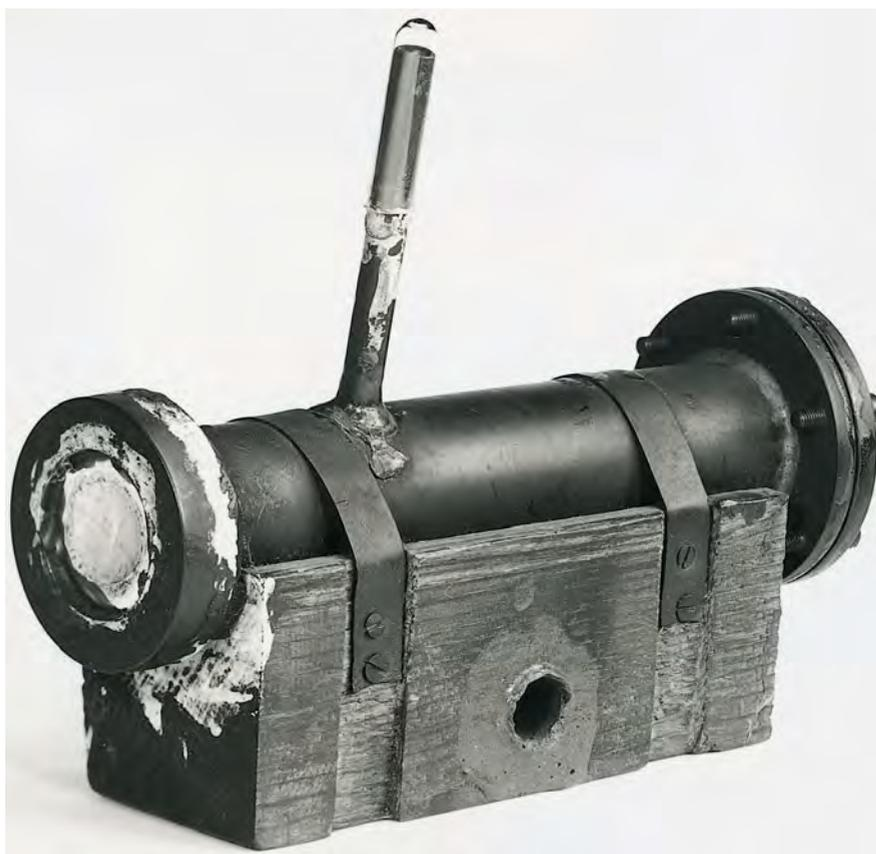
Fig. 2.23 Apparatus Chadwick used in his discovery of the neutron. Alpha particles from a polonium source, at the right end, bombarded a beryllium target at the left end. A penetrating, neutral radiation – neutrons – emerged from the beryllium.
