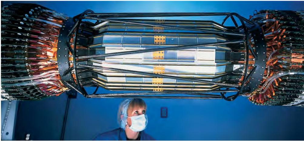
**Fig. 8.33** (TOP) The silicon strip detector that lies at the heart of the BaBar experiment at SLAC's PEP-II collider contains five concentric layers made up from 52 doubled-sided silicon strip detectors, with a total of 150 000 strips.
