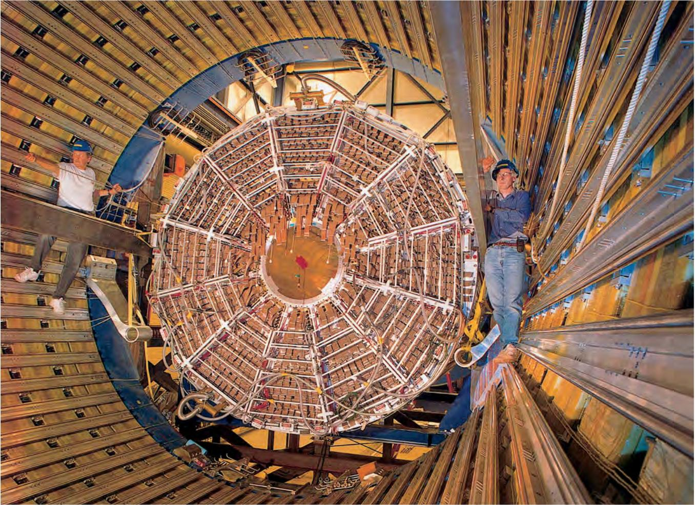
**Fig. 8.9** The world's largest time projection chamber is installed in the STAR experiment at Brookhaven National Laboratory's RHIC collider. Visible is one end of the 4.5 m long and 4 m diameter chamber as it is about to slide within the cylindrical electromagnet. The huge volume (53 cubic metres altogether) is divided into 12 segments at each end, where the ionization from charged particles traversing the chamber is detected.
