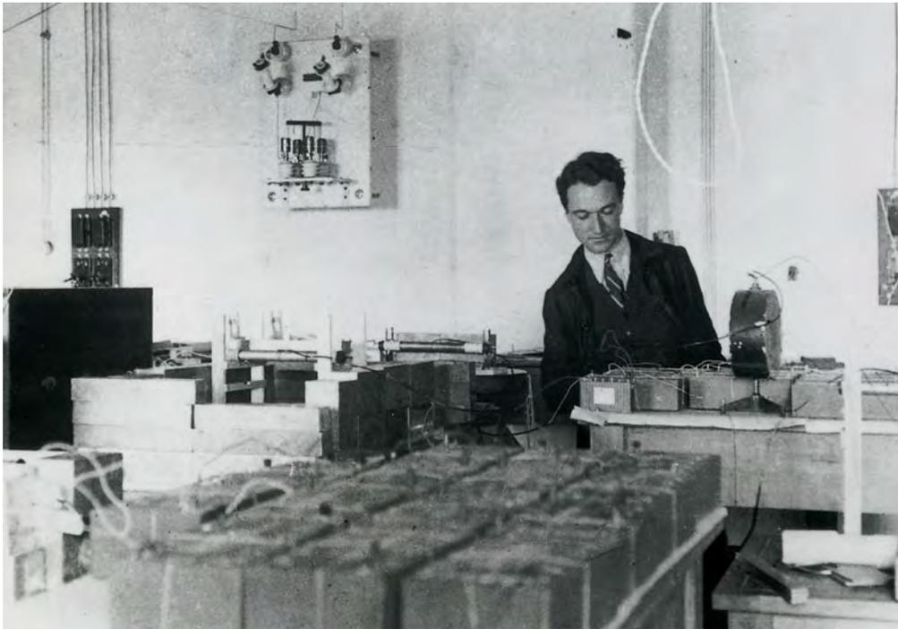
**Fig. 4.7** Bruno Rossi (1905–1993) working in his laboratory at the Physics Institute of the University of Florence, around 1930. The horizontal tubes just visible in the centre of the picture are Geiger–Müller counters. Ranks of dry cells (batteries) provided the high voltage for the counters.
