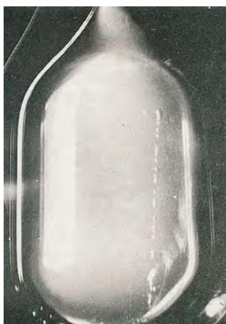
**Fig. 6.22** The track of a cosmic ray passes through Donald Glaser's first bubble chamber, a small glass phial holding a mere 3 cl of diethyl ether.
