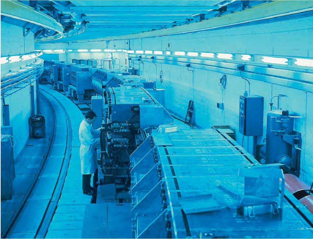
**Fig. 6.28** CERN's proton synchrotron – the 'PS' – accelerated its first protons to 24 GeV in 1959. The machine was later upgraded to run up to 28 GeV and today continues to form a vital part of a complex of interconnected machines that has accelerated beams of protons, antiprotons, electrons, positrons, and heavy ions.
