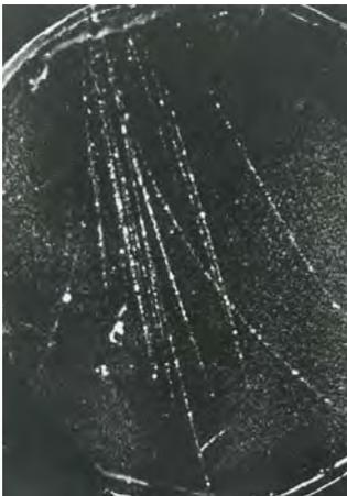
**Fig. 4.13** An image from the cloud chamber used by Blackett and Occhialini shows a 'shower' of electrons and positrons produced by a cosmic ray that has interacted in the wall of the chamber. The particles are clearly of opposite charge, bending in opposite directions in the chamber's magnetic field.
