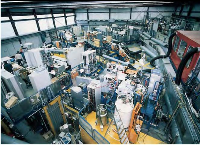
**Fig. 12.9** (LEFT) The HASYLAB area at DESY in Hamburg has many experiments crowded together to receive beams of X-rays and UV radiation produced by the synchrotron, DORIS III. This ‘synchrotron radiation’ is emitted by electrons or positrons in the machine as they follow sharply curving paths through special magnets, called ‘wiggler’ and ‘undulators’. Beams from DORIS III serve 42 experimental stations for research in areas from materials science and geology to medicine.
