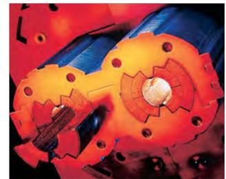
**Fig. 11.2** The LHC will contain two proton beams travelling in opposite directions but within a single ring of magnets. The magnets will have a novel '2-in-1' design, incorporating oppositely directed magnetic fields side by side, to control the oppositely curving beams. This engineering model shows the design of the superconducting dipoles – the bending magnets – with the two holes for the twin beam pipes for the counter-rotating beams.
