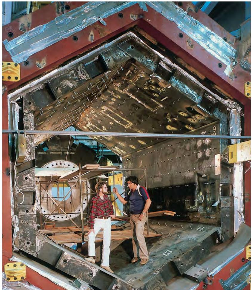
**Fig. 8.8** David Nygren, left, inventor of the time projection chamber, stands inside the hexagonal steel of the calorimeter that surrounded the 2 m diameter chamber built to study electron–positron collisions at the PEP collider at SLAC in the 1980s. The chamber was surrounded by the coil of a superconducting magnet, to bend the charged particle tracks.
