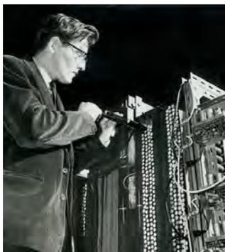
**Fig. 6.30** Fred Ashton at work on an array of flash tubes at Durham University. The glass tubes, seen end on, are a little more than 1.5 cm in diameter and are filled mainly with neon. They are stacked between metal plates, across which a high voltage is applied when a charged particle has passed through. The particle ionizes the gas in the tubes it crosses and they ‘flash’ under the influence of the electric field between the plates, revealing the path of the particle.
