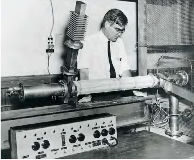
**Fig. 6.38** (LEFT) William Hansen (1909–1949) with a section of his first electron linear accelerator, which operated at Stanford University in 1947. It was 3.6 m long and could accelerate electrons to an energy of 6 MeV.
