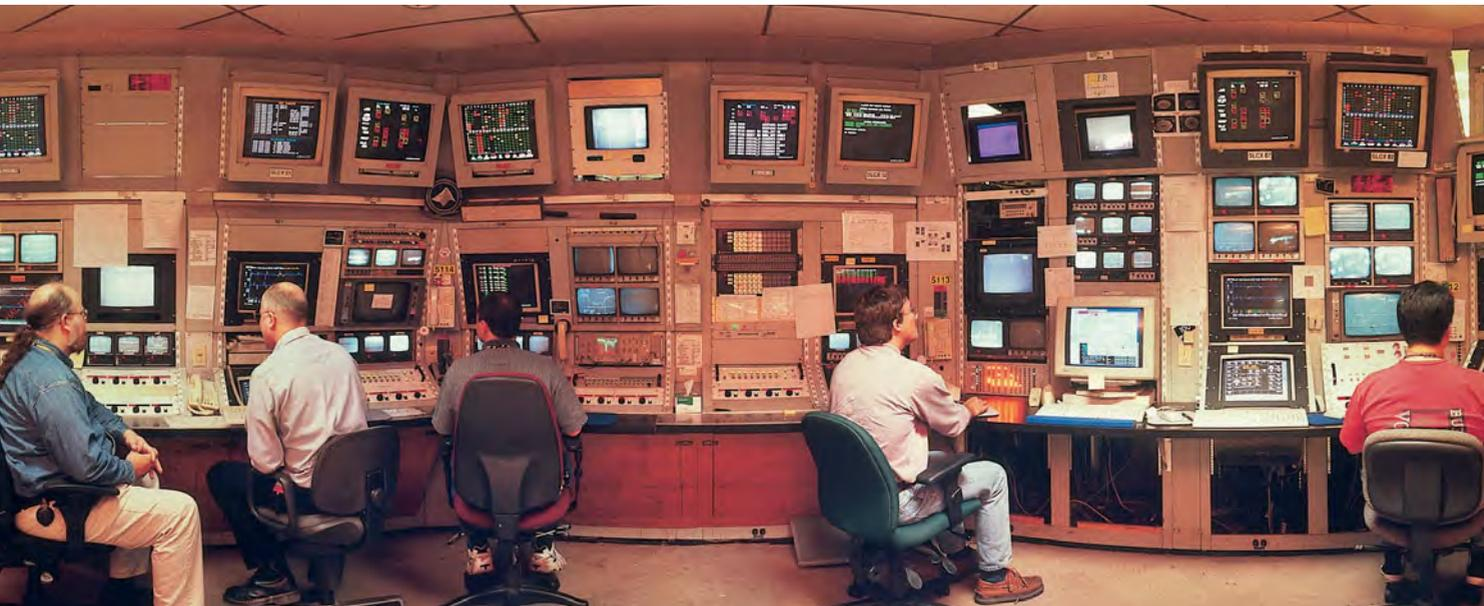
**Fig. 1.15** The control room is the nerve centre of a particle accelerator. In this image, banks of monitors show the status of key components in the various machines at the Stanford Linear Accelerator Center in California. The machine crew is in charge, ensuring that the accelerators deliver their beams as smoothly as in an industrial process.
