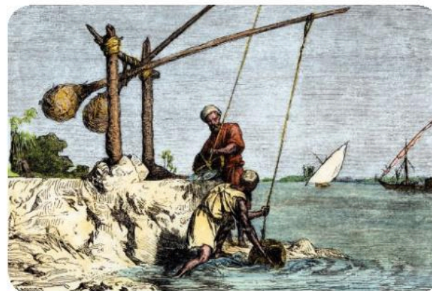
Ancient Egyptians using a shaduf to lift water from the River Nile
