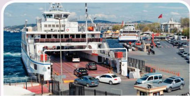
Roll-on roll-off ships have large doors at the bow (front) and stern (back), allowing cars and trucks to be driven straight on or off of the ship to load and offload cargo.
