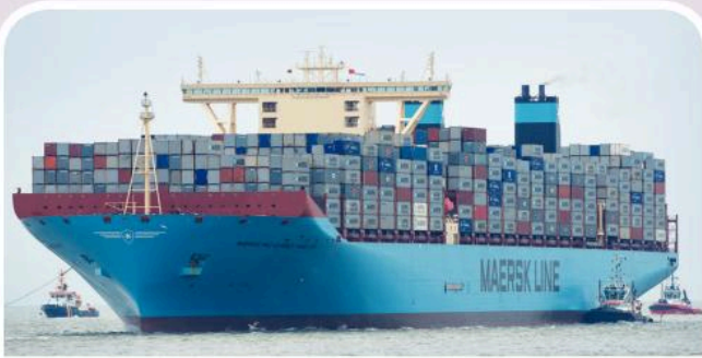
One of the world's largest container ships, the Marie Maersk , is 398 metres long and 58 metres wide, and can carry more than 18 000 containers.
