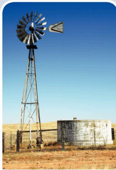
Wind pumps are used to lift water from wells and drainage ditches.
