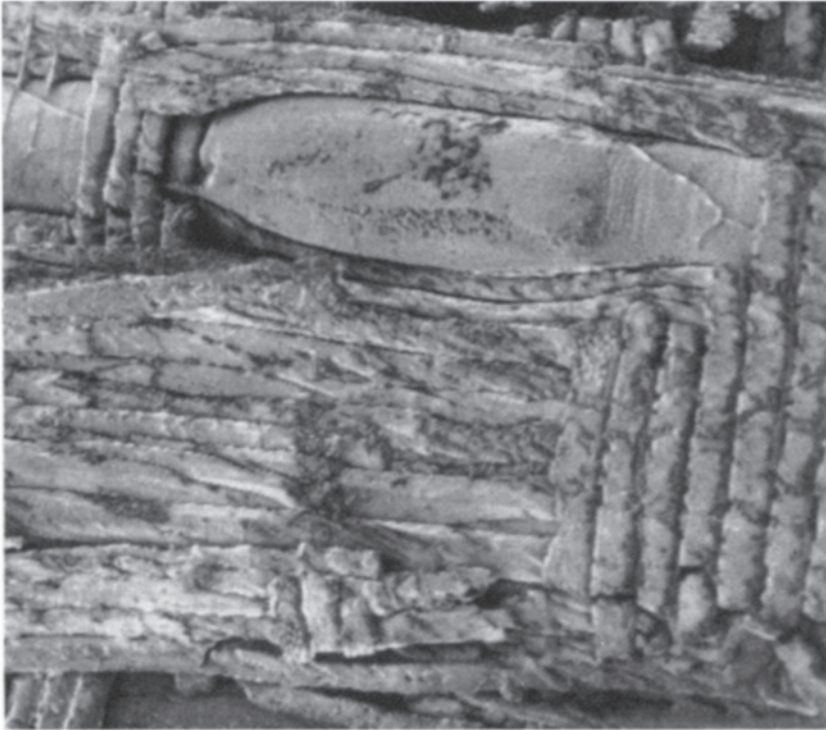
Plate 3.12 A scanning electron microphotograph showing wood replaced by iron corrosion products
