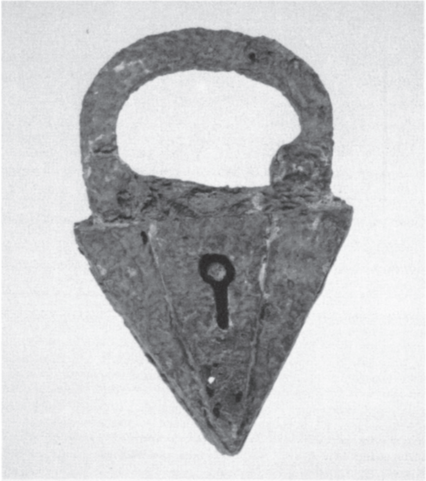
Plate 5.11 Careful mechanical investigative cleaning of ironwork reveals plating and original surface (cf. plate 1.3)
