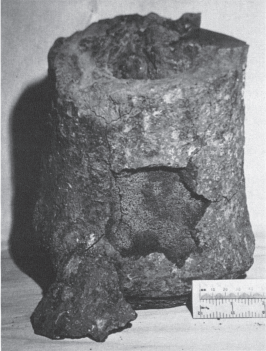
Plate 5.8 Part of a cannon retrieved from the sea where a fragment of the outer graphitized zone has broken away from the remaining cast iron core
