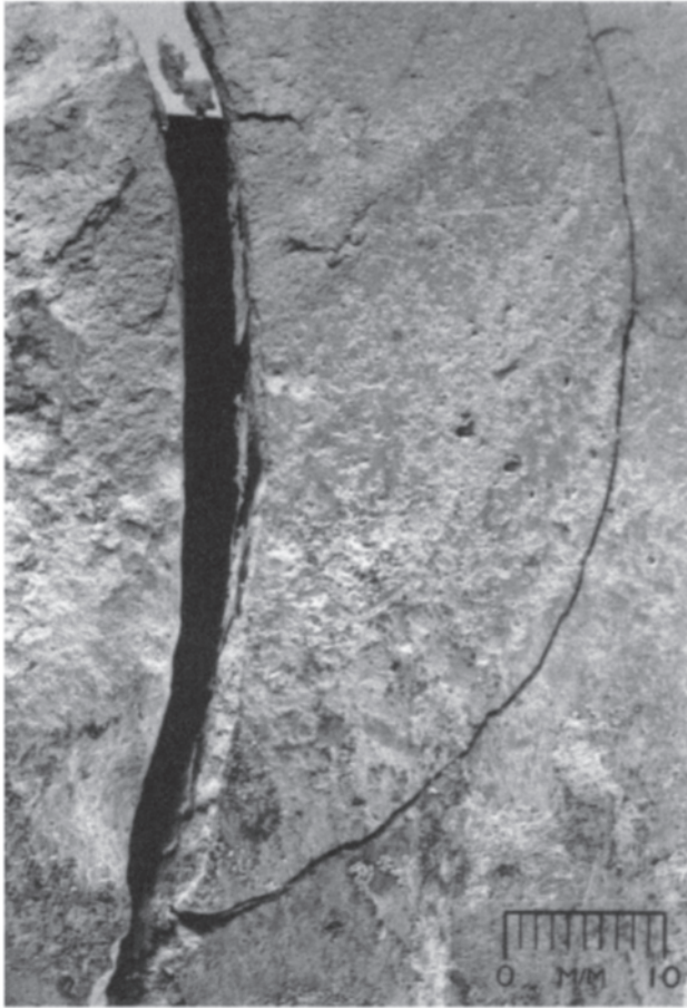
Plate 4.18 A join fails in a reconstructed ceramic as a result of the body powdering. A detached skin of adhesive and ceramic is visible
