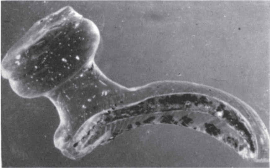
Plate 4.10 Iridescent glass, (a) Deteriorated glass showing iridescence, (b) The same glass immersed in a liquid which obliterates iridescence by displacing the air in the weathered surface
