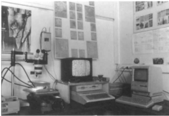
4.8 Apparatus for measuring tree-ring thicknesses. The screen in the centre of the photograph shows a series of rings from a sample mounted beneath a microscope and video camera on the left. Individual rings can be measured precisely and recorded by a microcomputer, while the more sophisticated computer on the right runs programs to match the series of measurements with sequences of known date. Laboratoire de ChronoEcologie de Besançon; photograph by Olivier Girardclos
