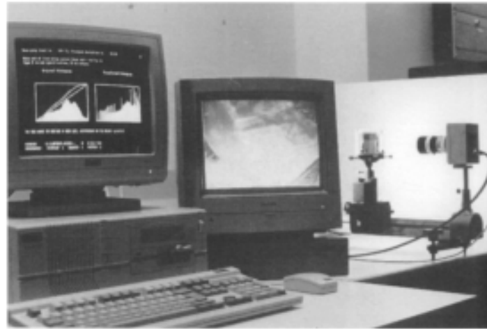
2.9 Aerial photographs may be digitized for computer analysis, and then processed by programs that filter out irrelevant background variations and enhance significant details. Oblique photographs can also be adjusted to compensate for distortions of angle, and matched precisely to maps. This illustration shows an inexpensive PC-based imaging system in which a video camera is examining a negative. The graphs on the left represent scales of tones found in the photograph; they can be altered to produce modified images on the other screen. Booth et al., 1992, fig. 27.1
