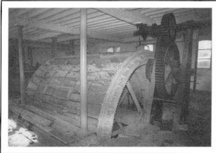
Plate 9 A rare survival, the breastshot waterwheel in situ at St Mary's Mill, Chalford, in Gloucestershire. The machinery of this former woollen mill was driven by gearing from the internal rim of the wheel and by an auxiliary Tangye steam engine which also survives.
