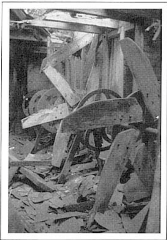
Plate 33 The scutching machinery in a derelict water-powered mill at Cleggan in Northern Ireland: the central iron rim and the wooden wiper blades, known as a scutching handle, would have been enclosed on one side to protect the operatives who held the bunches of flax against the rotating blades.
