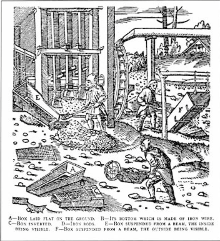
Figure 48 Agricola's illustration of a battery of water-powered ore stamps. He shows that the broken ore is passed through a series of sieves and the coarser material returned to the stamps for further reduction. The remains of similar boxes and sieves have been found on excavations of nineteenth-century metallic ore-processing sites, showing their continued use long after his sixteenth-century drawing.
