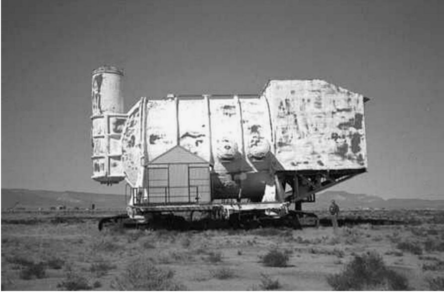
Figure 7.5 The test chamber used in the Huron King underground test. For scale, note the person standing under the right hand side of the chamber
