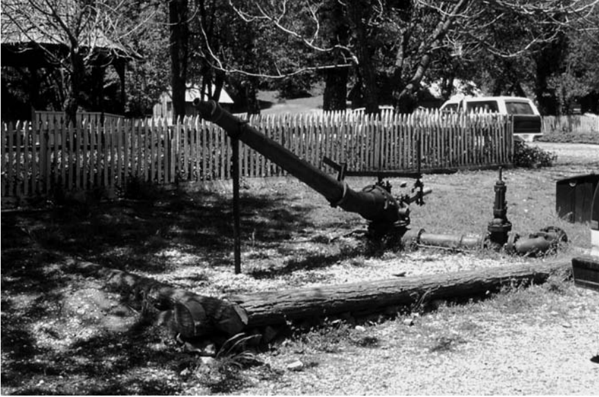
Figure 5.3 “Giant” water nozzles used for hydraulic mining in the mid-nineteenth century, Malakoff Diggings State Park, California
