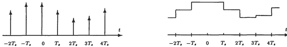
Fig. 3-7. The use of a zero-order hold to interpolate between the samples in x_s(t) .
