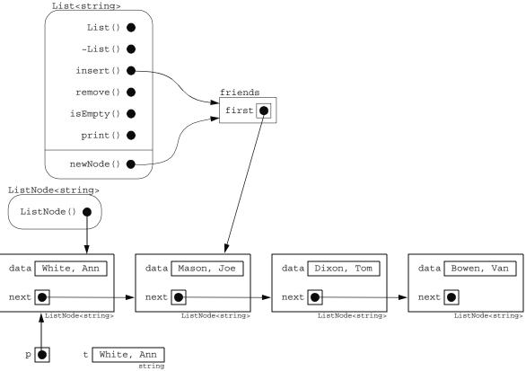
This shows the situation at the moment that the <code>insert()</code> function has invoked the <code>newNode()</code> function which has invoked the <code>ListNode()</code> constructor to create a new node for "White, Ann".
