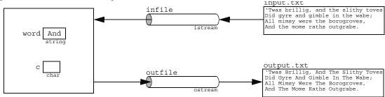
Notice that the program has four objects: an ifstream object named infile, an ofstream object named outfile, a string object named word, and a char object named c.
