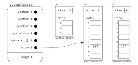
w, and x have been instantiated from the class. Note that the copy() function is a protected utility function, so it cannot be invoked by any of the class instances.
