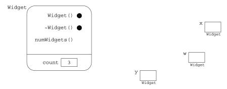
The difference is that now the member function <code>num()</code> has no "this" pointer. As a static member function, it is associated with the class itself, not with its instances.
