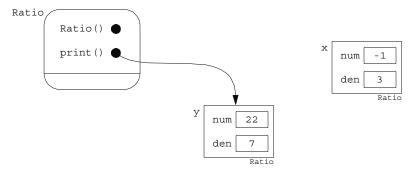
The class itself is represented by a rounded box containing its member functions. Each function maintains a pointer, named "this", which points to the object that is calling it. The snapshot here represents the status during the execution of the last line of the program, when the object y is calling the print() function: y.print(). At that moment, the "this" pointer for the constructor is NULL because it is not being called.
