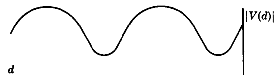
Fig. 8-6. Standing wave pattern on a lossless line, caused by a terminal load impedance that produces a reflection coefficient of magnitude about 0.4.
