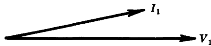
Fig. 4-4. Phasor diagram of the time-harmonic voltage and current at the input terminals (i.e. z = 0 ) of a transmission line terminated in its characteristic impedance. The phasors are related by V_1/I_1 = Z_0 .
