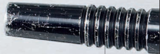
Rifle barrel has cooling fins
