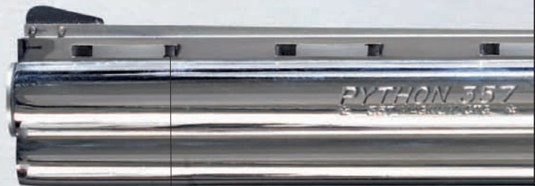
Ventilated barrel rib
