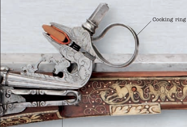
Spring holds cock firmly against striking wheel
