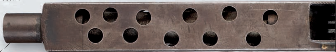
Perforated barrel shroud serves as the fore grip
