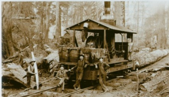
Loggers pose beside a "walking donkey," a steam engine for pulling logs down railroad tracks, Mason County, Washington, ca. 1901.
