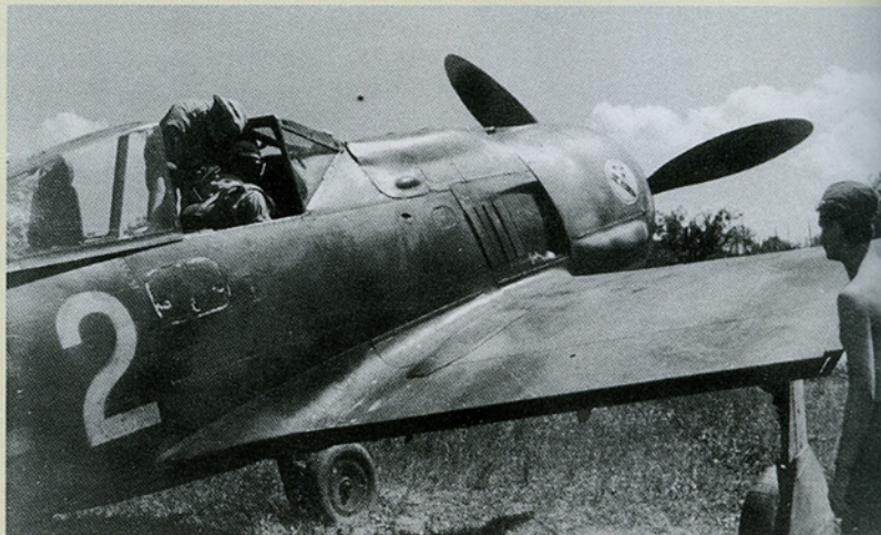
ABOVE: Ground crew of 1./SG 4 helping the pilot of 'White 2' strap in. Although this aircraft lacks head armour, a blown canopy and underwing bomb racks, it is thought that this is, in fact, an Fw 190 F-8, a version which was delivered to SG 4 in May 1944, shortly before the unit was withdrawn from the front due to its high losses. By this time the Luftwaffe's ground-attack units had phased out their earlier letter codes in favour of fighter-style markings.
