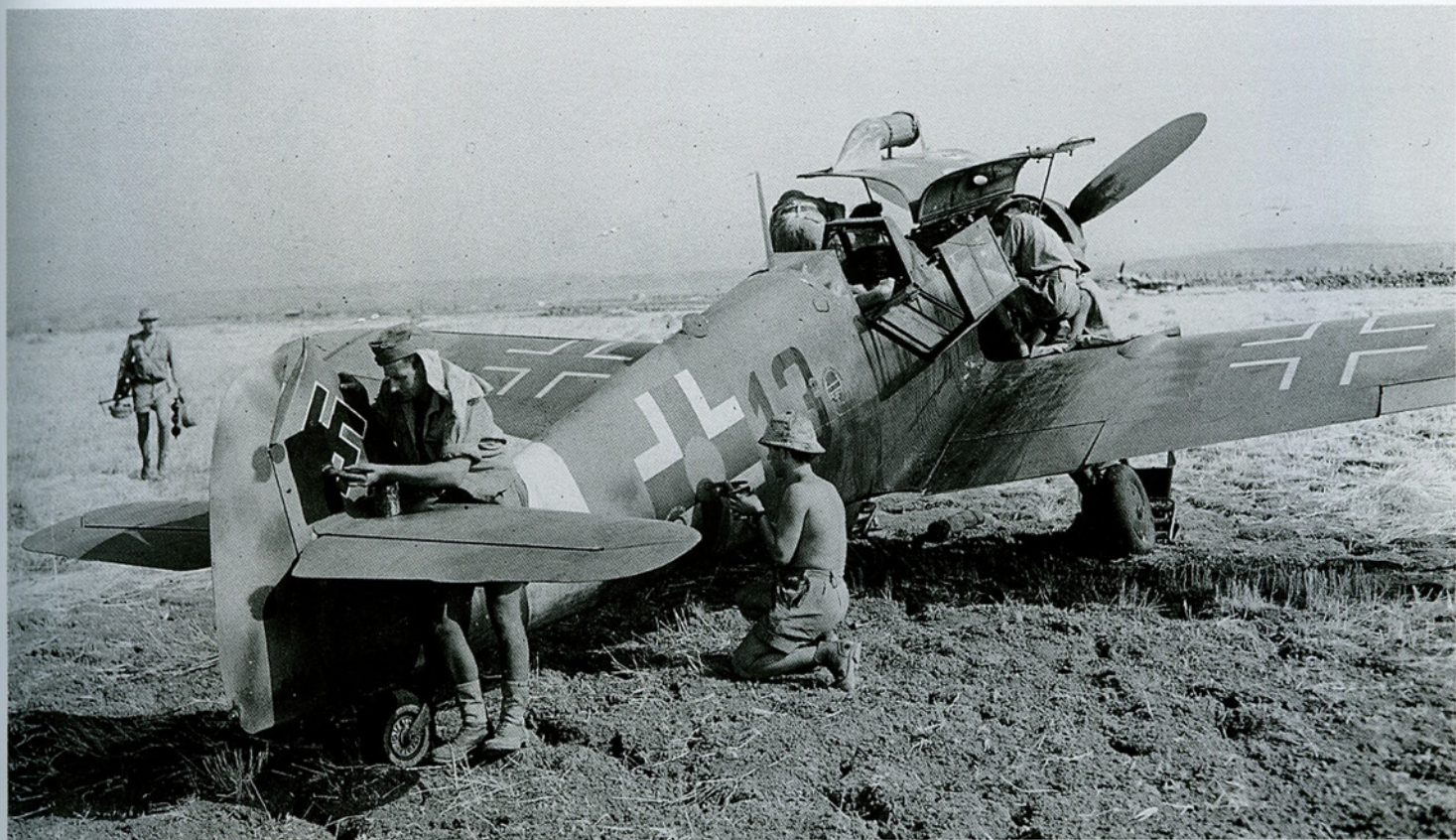
ABOVE: Allied personnel repairing and repainting an early Bf 109 G, 'Black 13' in RAF markings probably on one of the Gerbini group of airfields inland from Catania, in Sicily. Note the serrated demarcation between the uppersurface colours of the wings and tailplane and that the paint on the rear face of the propeller blade had been worn away. Unfortunately, no details of this aircraft have been located in Allied Intelligence reports.
