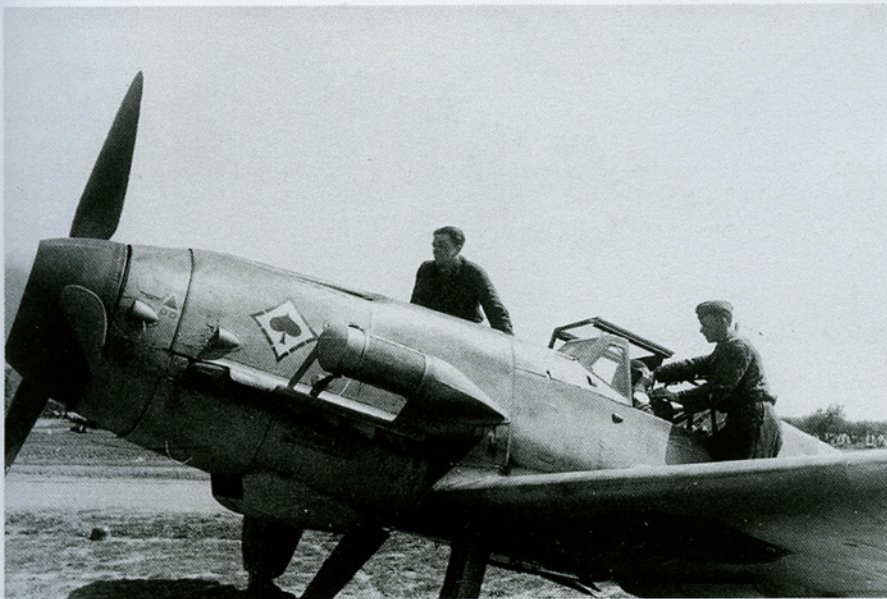
LEFT: A Bf 109 G-2/trop of JG 53. Clearly visible in front of the supercharger intake is the air cleaner fitted to tropicalised versions of the aircraft. This air cleaner consisted of two Delbag air filter units and two switchover flaps which were operated by cable from a hand lever on the left hand side of the cockpit. The Delbag filter units removed impurities from the air by means of a thin coating of oil, and because they soon became choked, they had to be changed or cleaned after every two flights. The cleaning was achieved by dipping the filters in a solvent, such as petrol or paraffin, etc, and allowing them to dry. They were then re-dipped in used engine oil and allowed to drain.
