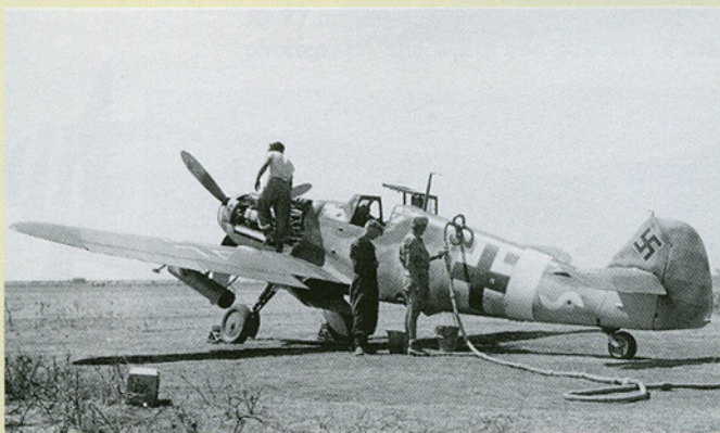
Once armed, the 400 litre fuselage fuel tank of 'Yellow 14' is refilled (ABOVE) and the engine started (RIGHT). The full Stammkennzeichen and Werk Number of this machine are believed to have been RH+JD, which was retained below the wings, and 15762 respectively.
