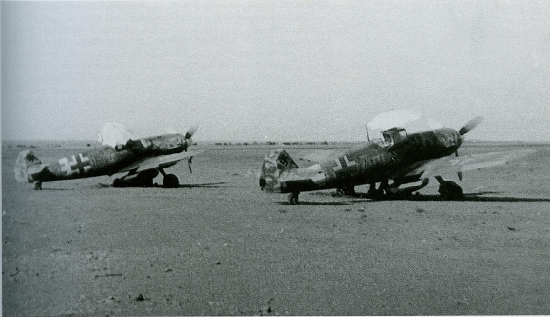
LEFT: Photographed at Tanagra in the summer of 1943, these Bf 109 G-6s, 'Yellow 7' and 'Yellow 15', belonged to 12./JG 27, a Staffel which, when a IV. Gruppe was added to the Geschwader in May 1943, had been created by redesignating the former 8. Staffel. Both machines are finished in standard grey RLM 74/75/76 camouflage colours, and while the white theatre bands around the rear fuselage have been retained, the earlier white rudders have been toned down with an overspray of darker camouflage colours. Just visible on 'Yellow 15', furthest from the camera, is the double horizontal bar symbol adopted by IV./JG 27 as a Gruppe identification. The yellow numerals on these aircraft have been outlined thinly in black.
