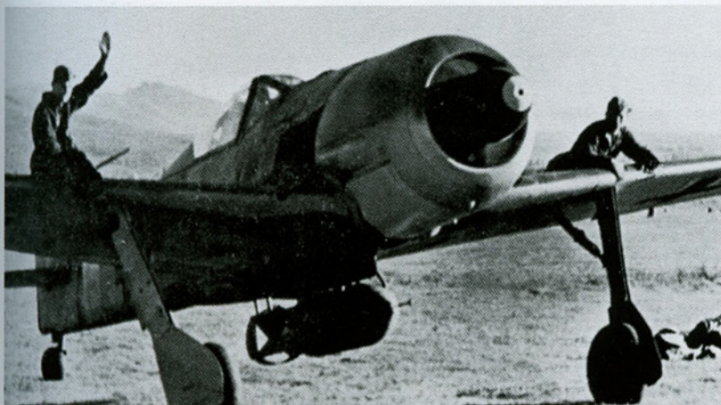
RIGHT: An Fw 190 of II. or III./SKG 10 in Italy in September or early October 1943, shortly before these Gruppen were redesignated and formed parts of SG 4. Note that only the fuselage centreline rack carries a bomb, the two wing fairings for drop tanks being left empty as, although the extra fuel increased the aircraft's range, the tanks were generally disliked and little used because of the effect on the aircraft's speed. On one earlier occasion, when SKG 10 was ordered to mount an operation from southern Italy against targets in Tunisia, the weight of the two tanks was such that no bomb was carried and the attack was carried out using only the aircraft's cannon and machine gun armament.
