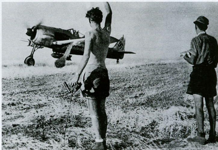
RIGHT: An Fw 190 of II. or III./SKG 10 in Italy in September or early October 1943, shortly before these Gruppen were redesignated and formed parts of SG 4. Note that only the fuselage centreline rack carries a bomb, the two wing fairings for drop tanks being left empty as, although the extra fuel increased the aircraft's range, the tanks were generally disliked and little used because of the effect on the aircraft's speed. On one earlier occasion, when SKG 10 was ordered to mount an operation from southern Italy against targets in Tunisia, the weight of the two tanks was such that no bomb was carried and the attack was carried out using only the aircraft's cannon and machine gun armament.
