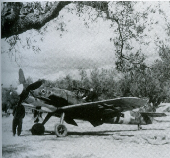
LEFT AND ABOVE: These two Bf 109 G-4s belonged to II./JG 53 and were probably photographed in Sicily in May or June 1943. Both machines have a similar uppersurface camouflage consisting of a low demarcation RLM 79 desert sand colour, over which has been sprayed a dark green pattern similar to the so-called Wellenmuster or wave pattern finish.
