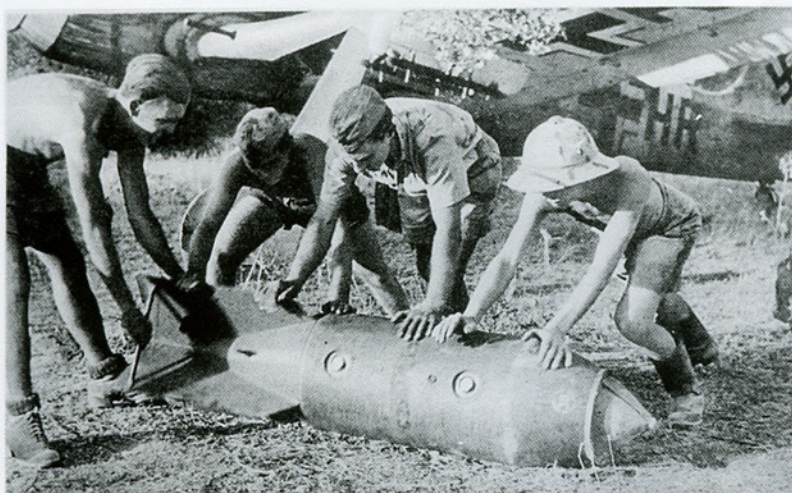
ABOVE: An operational Fw 190, clearly still wearing its Stammkennzeichen, being bombed up. This particular example is believed to be a G-3, probably DP+HR, W.Nr. 160044. Note that the wing racks, which allowed this aircraft to carry drop tanks or bombs, were rarely used in Sicily and Italy and were frequently removed.
