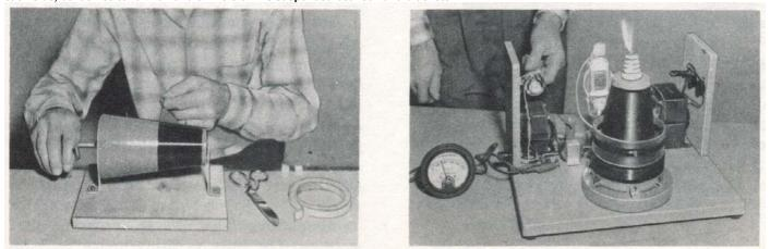
After you finish the assembly, read the plate current by connecting a D.C. milliammeter between the center tap of the filament transformer and ground. Adjust the rheostat to 150 ma. maximum for any combination of capacitors and taps
