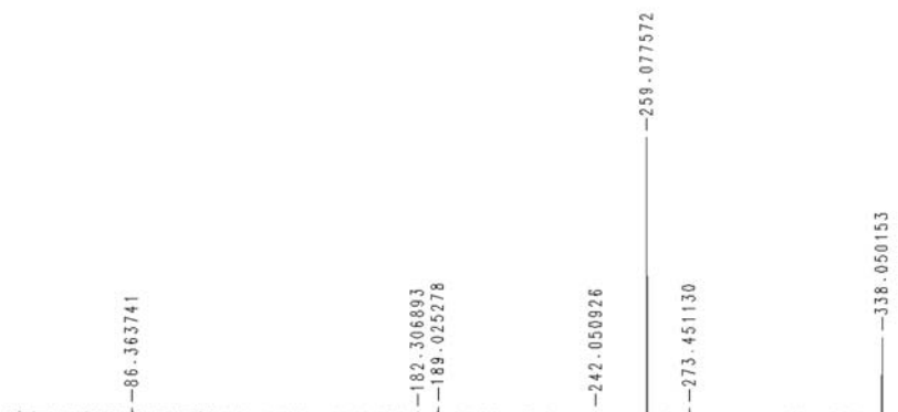
FIGURE 33 FTMS/MS daughter ion mass spectrum of the API in the counterfeit tablets.
