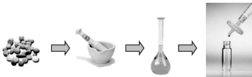
FIGURE 1 The common sequence of sample preparation steps for drug products: grinding → extraction → dilution → filtration.
