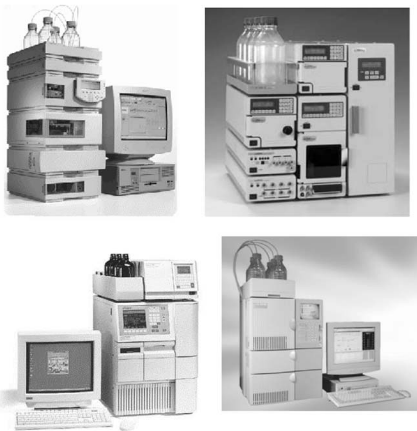
FIGURE 2 Examples of modular and integrated HPLC systems. Upper row (l to r) modular systems: Agilent 1100 Series, Jasco LC-2000 Series; Lower row (l to r) integrated systems: Waters Alliance, Shimadzu LC-2010.
