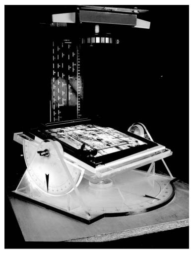
**Figure 6.6** Rectification table used to rectify photographs under an enlarger. Most darkroom techniques have now been replaced with digital imagery, particularly the rectification of tilt can be managed more quickly and efficiently with programs like Photoshop rather than the cumbersome and time-consuming darkroom methods.
