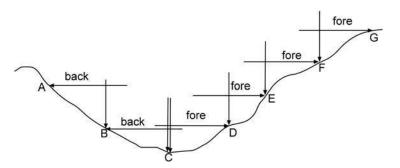
**Figure 4.16** Back and fore readings. This shows the process from point A to point G with fore and back readings using the modified builders level shown in Figure 4.12(c).
