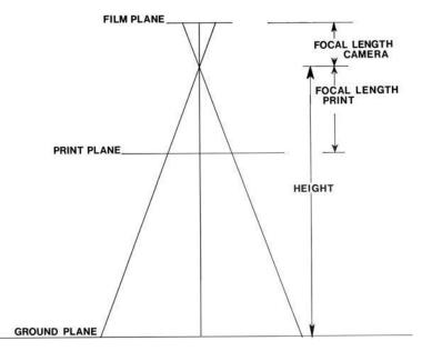
**Figure 6.3** Schematic showing the main distances involved in photography. The image shows the relative position of the negative, the center of the camera lens, the plane of the print, and the plane of the object. Knowing the focal length of the camera lens allows the calculation of angles and sizes of objects in any of the planes.
