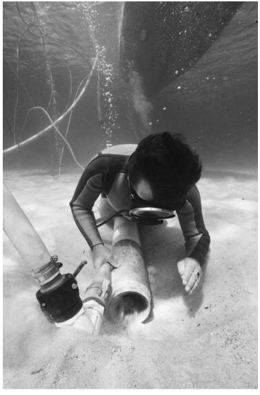
Figure 9.13 Working end of a water dredge showing where high-pressure water is injected into the dredge head. (Courtesy of Patrick Baker, Department of Maritime Archaeology, Western Australian Maritime Museum.)
