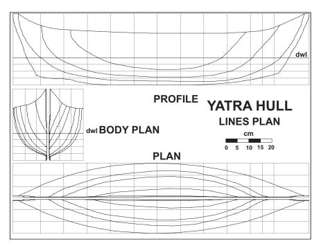
**Figure 11.16** Line drawing of a *Yatra Dhoni* in Sri Lanka. The line drawing enables naval architects to make calculations about the performance and capacity of the vessel. This plan is used in the construction of the vessel. (Courtesy of Brian Richards, Department of Marine Archaeology, Western Australian Maritime Museum.)
