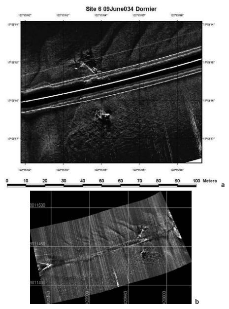
**Figure 3.36** Side scan sonar target displayed as a GeoTIFF. Note the sonar trace in (a) is geographically coordinated by the processing software but does not allow for the removal of the water column (the dark center line). In this case positions on the GeoTIFF are not strictly correct (pseudo-georeferenced). In case (b) using SonarWeb, the processing has removed the water column thus allowing for slope correction. Any position on this GeoTIFF will be correctly georeferenced.
