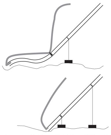
**Figure 9.10** Two types of airlift design, one with a flexible hose and rigid riser and the other rigid.
