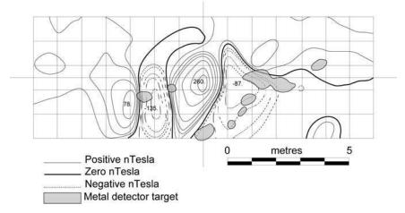
**Figure 5.2** Magnetic close-plot survey in Kyrenia showing the metal detector survey superimposed on the contour plan. Shaded areas indicate metal detector targets. Z1 and Z4 correspond to magnetic anomalies whereas other metal detector targets do not correspond to magnetic targets. This indicates nonferrous targets. Subsequent excavation showed these targets were lead sheathing.
