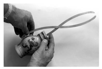
Figure 11.4 X-calipers used to measure the wall thickness inside jars and pots. The calipers are set so that the gap is identical at each end of the caliper.
