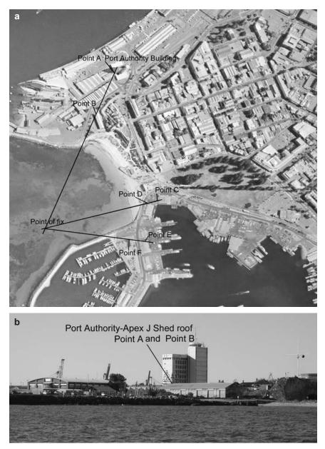
**Figure 3.2** Photo transits and how they work. Four illustrations include an aerial photograph (a) and three transit photographs (b), (c), and (d). Figure 3.2b shows the alignment of the Port Authority Building (A) with the apex of the roof of J Shed (B). This line can be seen on Figure 3.2a.
