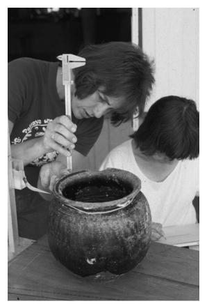
**Figure 11.8** Profiling device used to measure the shape of a large object. In this case the X and Y coordinates are read off the scales on the profiler and transferred to the artifact drawing. (Courtesy of Brian Richards, Department of Maritime Archaeology, Western Australian Maritime Museum.)
