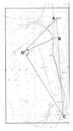
**Figure 3.7** Sounding sextant fundamentals. This figure shows how the two included angles, AOB and BOC, which are the angles between Woodman Lighthouse (A) and the Obelisk (B) and the Obelisk and the 193-m high chimney (C) at the Alcoa Aluminum Refinery (all prominent features), are used to locate the position of the survey vessel.
