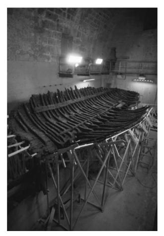
**Figure 13.2** The reconstruction of the original timbers of the Kyrenia ship, Cyprus, following excavation and conservation. This was the first time a complete excavation involving the dismantling of a wreck site culminated in the rebuilding of the vessel.
