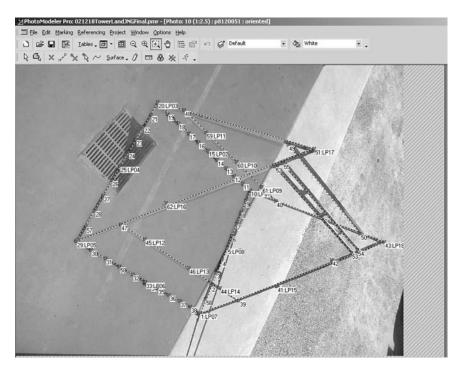
Figure 4.27 Photo tower on land shown in the mark-up mode of PhotoModeler interface.
