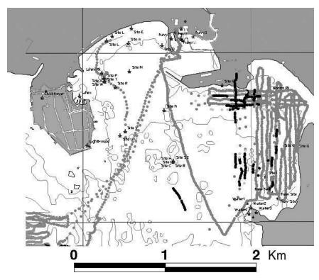
Figure 7.5 Plot of a search pattern in Galle Harbour, Sri Lanka, on a GIS.
