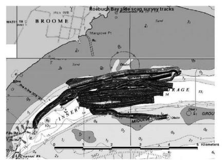
**Figure 3.37** Side scan mosaic Roebuck Bay, Western Australia. The sonar mosaics have been created from converting sonar traces to GeoTIFFs and then placing them on the chart of the area.
