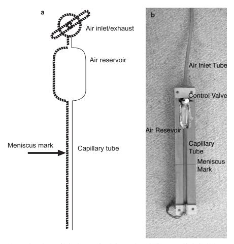
**Figure 4.15** The Martin depth-measuring device. A schematic diagram of this device is shown in (a) and a working version in (b). The device has a reservoir of air and a capillary tube. It is filled with air at depth so that the meniscus sits in the capillary tube. The device can be moved around at the same level to measure distances to objects.
