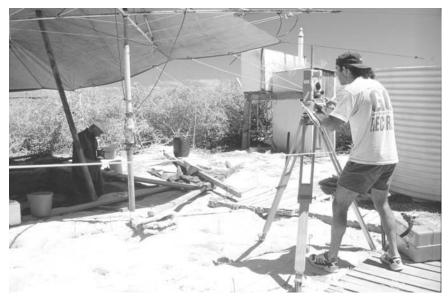
**Figure 3.13** A Total Station in operation. Note the operator on the left is holding a reflector that has been placed over a position to be recorded. The Total Station determines the distance and the azimuth of this point, recording these data electronically for later downloading. (Courtesy of Jochen Franke.)
