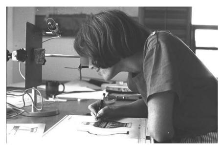
**Figure 11.6** Tracing device known as an Aerial Sketchmaster. Used mainly for photogrammetry, it can also be adapted to draw small artifacts. The instrument is set so the operator looks through a prism and can sketch the image on the paper below. The scale is usually set at 1:1.
