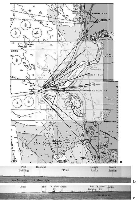
**Figure 3.11** Photo resectioning using an overlay (a). This can be used to plot positions from photo triangulation or from any other angle-measuring system. Note that the angles that are used in (a) are obtained from figures (b) and (c). The angles are calculated from knowing the focal length of the camera lens and the frame format as shown in Figure 3.3. The calculated angles are drawn on a sheet of clear film and adjusted over the chart to obtain the position.
