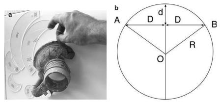
Figure 11.9 (a) Curvature measurement using fixed curves. (b) Basics of calculating the radius of curvature.
