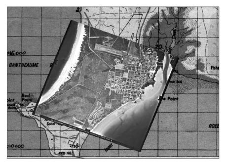
**Figure 7.4** Georeferenced historical map. In this example an aerial photograph of Broome, Western Australia, is linked to a topographical map by georeferencing.
