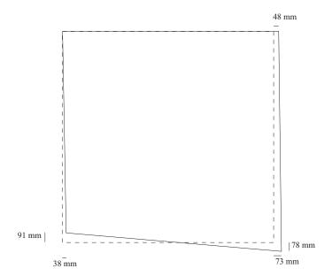
Figure 4.26 Example of HPASS measurement of a 2-m grid square on the Pandora site.
