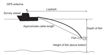
**Figure 3.28** A schematic showing the principle of layback. Cable equations are complex, but an estimation of the horizontal distance from the detector head behind the boat is important when conducting accurate surveys.
