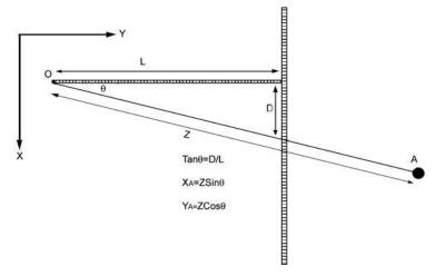
**Figure 4.2** T-shaped angle-measuring device. This is more accurate than the protractor. In this case the angle is determined from the arctan ratio of D/L.
