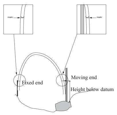
**Figure 4.14** Static bubble tube has a fixed volume of air in tube, and one end (the fixed end) is brought to a fixed datum point and the meniscus point marked on the working end. The measuring end can then be used to measure from meniscus to object.
