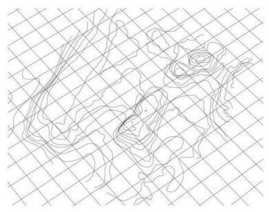
**Figure 6.17** A contour plan of the Tektash site made from stereophotographs and then imported into Rhino to produce a three-dimensional plan.
