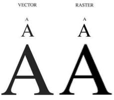
**Figure 7.2** Enlargement of vector and raster graphics. Image on left shows vector graphics image of letter A at three different enlargement sizes. On the right is shown the same images in raster format. The vector image can be enlarged indefinitely without loosing line quality.
