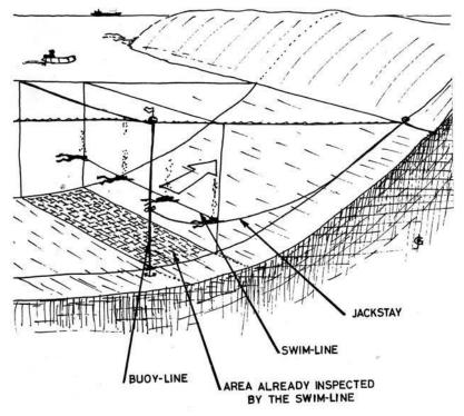
**Figure 3.17** Swimline schematic at Cape Andreas, Cyprus, showing four divers holding the swimline and the first diver following the jackstay. The team has been deployed from the boat at the surface starting from the buoy at the buoy line.
