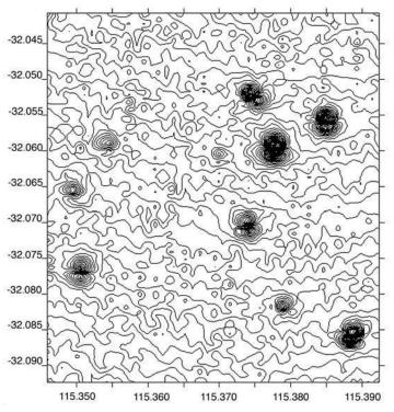
**Figure 3.26** Contour magnetic map. This map was generated from an aerial magnetic survey of the Deepwater Graveyard off the Western Australian coast, an area off the port of Fremantle where ships were scuttled. Water depth ranges between 80 and 100 m.
