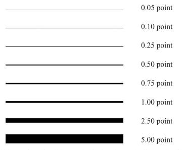
Figure 11.1 A series of line thicknesses showing how the very fine lines tend to disappear.
