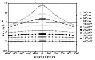
**Figure 3.30** Plot of the theoretical field intensity (logarithmic scale) against different ranges from the center of the anomaly for different depths of water in meters (mW).
