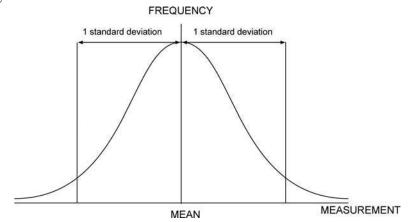
Figure 4.29 A typical normal or Gaussian distribution.
