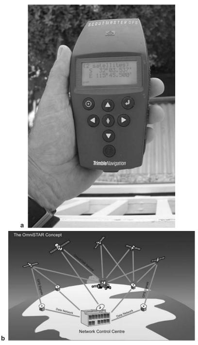
**Figure 3.14** (a) A hand-held GPS unit. (b) A schematic showing how a DGPS system works, in this case the satellite-based OmniSTAR system. The OmniSTAR satellite (second on left) is sent data from the Network Control Center which are broadcast to the remote receiver. These satellite data provide the GPS system with information allowing the GPS to operate in differential mode. (Figure 3.14b is courtesy of OmniStar, Fugro International.)
