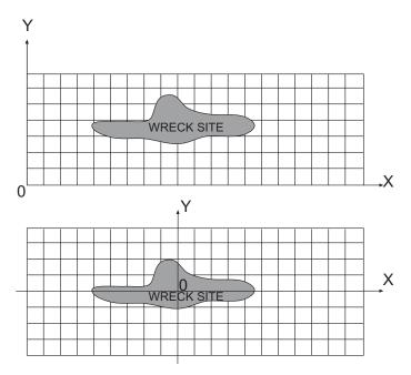
**Figure 10.4** A schematic showing two different types of grid coordinates. In the upper version the origin is centered off the site so all X and Y coordinates are positive. In the lower example the origin is in the center of the site creating positive and negative X and Y coordinates.
