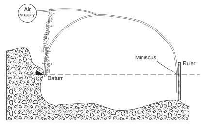
**Figure 4.13** Active bubble tube has air slowly bubbling through the tube. The point at which the bubbles stop coming out of one end and start coming out of the other end means the ends of the tube are level.
