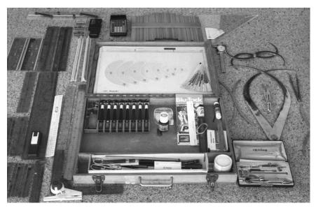
**Figure 11.3** A standard drawing box showing the range of equipment generally required for artifact and general site plan drawings.
