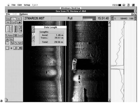
**Figure 3.34** Side scan sonar interface. This is the Marine Sonics side scan interface showing the standard display (a) with the size of object dialog box (showing length of wreck as 20.56m) and magnetometer trace along the right-hand side of the screen. The height of a target display interface (b) and a close-up image of the barge (c) seen in (a). (Figures 3.34a and b are courtesy of Eric Danielsen, Inwood (International) Pty Ltd.)
