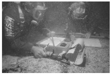
**Figure 4.19** HPASS diver unit. Operator on left is holding the mobile recording transponder. (Courtesy of Gary Cranitch, Queensland Museum.)
