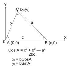
**Figure 4.5** Diagram showing how to solve trilateration. Point C, with coordinates  $x_3$ ,  $y_3$ , can be located if distances a, b, and c are known.
