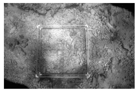
**Figure 6.1** Cross-hairs grid frame used to ensure vertical photograph. The photographer attempts to align the cross-hairs on the grid frame thus ensuring the camera is vertically above the frame.
