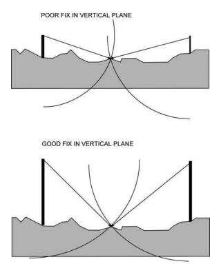
**Figure 4.11** Vertical control problems. Note that where there is little vertical elevation the fix is bad. With elevated control points the fix is improved, but constructing elevated control is often difficult. See Figure 6.13 where artificial control has been used.
