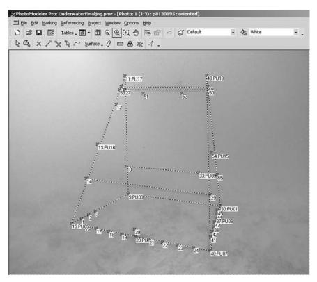
Figure 4.28 Photo tower under water, showing the mark-up mode of PhotoModeler interface.
