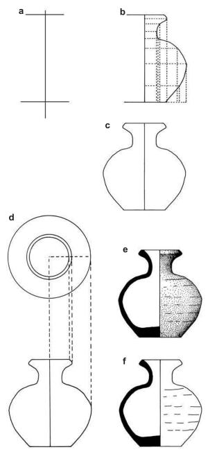
Figure 11.10 Stages of drawing a small jar showing the views and the construction method.
