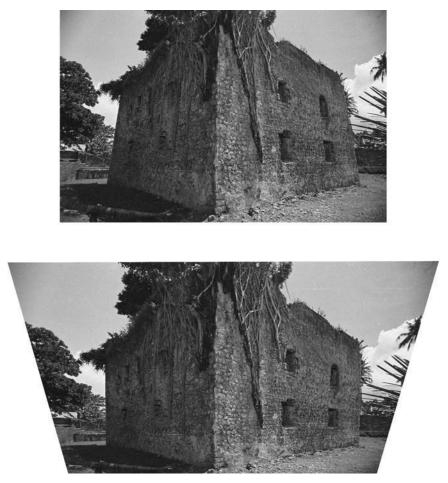
**Figure 12.2** Picture showing perspective distortion of a fort in Hila Ambon, Indonesia, and the correction of this distortion using a computer graphics package.
