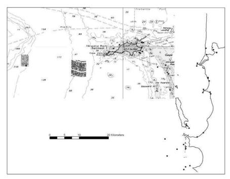
**Figure 3.29** A GIS of the Deepwater Graveyard showing the magnetic contour diagram shown in Figure 3.27 georeferenced on a chart of the area together with other data.
