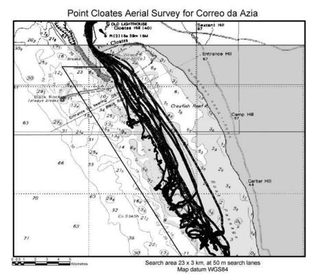
**Figure 3.19** *Correio da Azia* towed search in the Ningaloo Reef, Western Australia, showing the track of the search vessel recorded by GPS and then plotted on a chart using a GIS. Because the area consists of large coral heads (bommies), it is very difficult to search the area systematically. The GPS provides a good record of what areas have been covered and what need to be covered.
