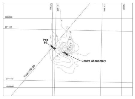
**Figure 3.27** Example of a magnetic survey conducted from a vessel over a geomagnetic anomaly, thought at first to be a World War II wreck site.
