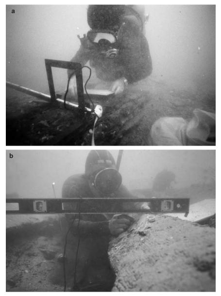
**Figure 4.12** Three simple profiling devices. (a) A horizontal bar with a right-angle frame used to measure profiles, the angle of the bar is horizontal and measured separately. (b) A carpenter's level used to measure from horizontal.
