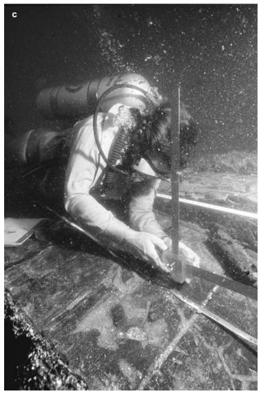
**Figure 4.12** (*Continued*) (c) A modified carpenter's level with bubble levels in two planes used to take vertical and horizontal measurements. (Figures 4.12a and c are courtesy of Brian Richards and Figure 4.12b is courtesy of Patrick Baker, both of the Department of Maritime Archaeology, Western Australian Maritime Museum.)
