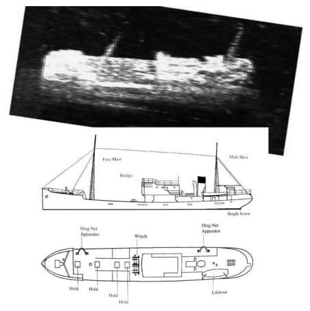
**Figure 3.35** Side scan sonar trace *Sapporo Maru* at Chuuk Lagoon in the Federated States of Micronesia. This illustration shows the sonar trace set against the scaled plan of the ship. From the sonar record it was possible to positively identify the ship before diving on it.
