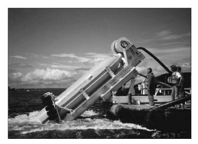
**Figure 3.32** A Fugro Seafloor Survey SYS 09 swath bathymetry side scan or multibeam sonar. This large-scale system produces accurate bathymetry by measuring the angle at which the seafloor reflections arrive at the stabilized and towed hydrophone array.
