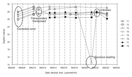
Figure 4.23 Corrected depth measurements on the Pandora site.
