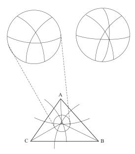
**Figure 3.3** Resectioning showing the "cocked-hat" effect, where the arcs represent distance measurements from three fixed points A, B, and C. Because at least one measurement is slightly wrong, the result is a cocked hat. If four points were used and only one measurement was wrong, the result would be as shown in the second enlargement.
