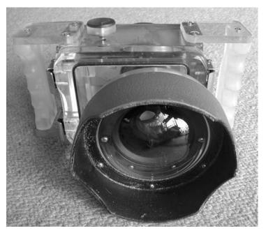
**Figure 6.16** UW digital camera. This system is an Olympus Camedia 3000 camera mounted in a custom-built Wills camera housing.
