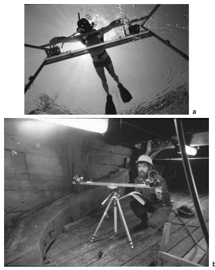
**Figure 8.2** Stereo camera bar on an underwater photo tower (a) and in a terrestrial situation (b) inside the *Wasa* at the Wasamuseet in Stockholm. Note in A the underwater cameras are mounted on small hand-held camera bars that are then attached to the stereo bars. (Figure 8.2a is courtesy of Patrick Baker, Department of Maritime Archaeology, Western Australian Maritime Museum.)
