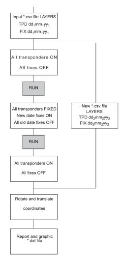
Figure 4.24 Flowchart of HPASS operation.
