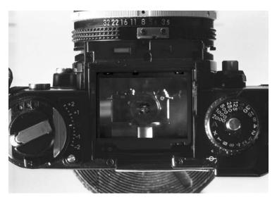
**Figure 12.6** Optical alignment of the camera. In this view we are looking into the viewfinder of the camera that has been set up perpendicular to the object plane. A small mirror, seen in this view, is used to ensure that the camera is exactly perpendicular to the object plane. (Courtesy of Brian Richards, Department of Maritime Archaeology, Western Australian Maritime Museum.)
