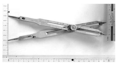
Figure 11.5 Proportional dividers used to scale measurements. The dividers have the common proportional measurements set so that the proportionality ratio can be set.
