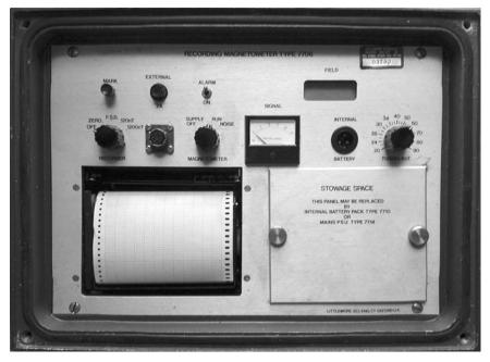
**Figure 3.25** The control unit of an ELSEC Small Boats Magnetometer EL7706. Magnetometer controls left to right central row above chart recorder: recorder control, RS232 data output, magnetometer control, signal strength meter, external power supply, and magnetometer tuning control. LCD window above external battery gives digital readout of magnetic field strength.
