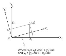
**Figure 4.6** Coordinate rotation showing how a coordinate system  $X_2$ ,  $Y_2$  is rotated to coordinate system  $X_1$ ,  $Y_1$ .
