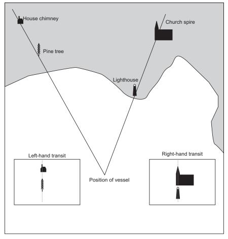
**Figure 3.1** Diagram showing how two or more visual coincidences (transits) enable one to locate position. In some cases if the objects used in the transits can be identified on a map or aerial photograph, then it is possible to plot position on a map. However, in general, transits are used at sea to locate position.
