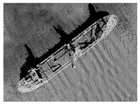
**Figure 3.33** Multibeam image of a shipwreck in the Persian Gulf. Data collected by the RESON SeaBat Multibeam System. (Courtesy of RESON.)
