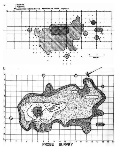
**Figure 5.4** Probe survey: (a) Kyrenia and (b) Cape Andreas. The simpler Kyrenia survey indicates the extent of the site, whereas the more thorough Cape Andreas survey indicates the depth of burial.
