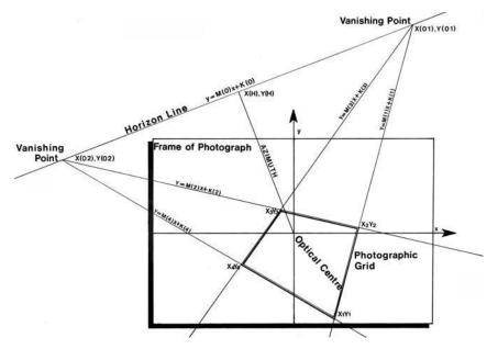
Figure 6.7 The general factors involving tilt in a perspective view of a square grid frame.
