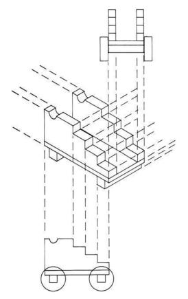
Figure 11.15 Drawing showing the basics of an isometric. In this case, a gun carriage is shown.
