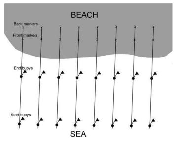
**Figure 3.6** Artificial transit network on a beach. This is a schematic showing how control points can be set up on a beach to provide visual transits for a boat operator so that regular search lanes can be steered. It is a simple and easy system to implement provided one is not too far offshore.
