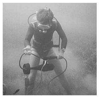
**Figure 5.1** Operator using nonferrous diving equipment to conduct a close-plot magnetometer survey on the Kyrenia wreck site. See Figure 5.2. (Courtesy of Kyrenia Wreck Excavation.)
