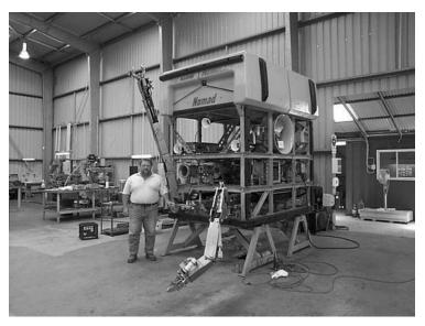
Figure 3.21 Large-scale ROV, the Nomad, produced by Total Marine Technology. (Courtesy of Tom Pado, Total Marine Technology.)
