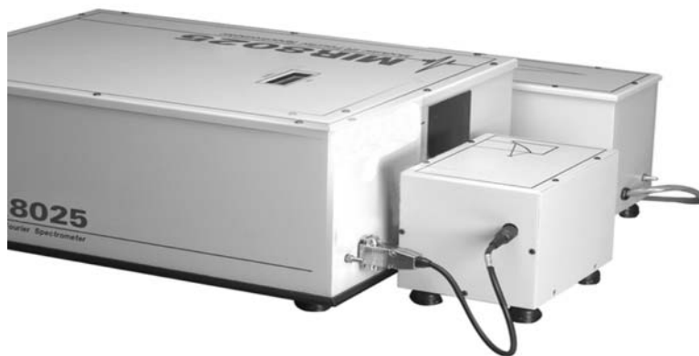
Figure 6.6 A deuterated triglycine sulfate (DTGS) detector for a mid-infrared spectrometer that exhibits large and spontaneous electrical polarization signals when the incident infrared beam affects its polarization. Permission to use this photo has been granted by Newport Corporation. All rights reserved ( www.newport.com ).
