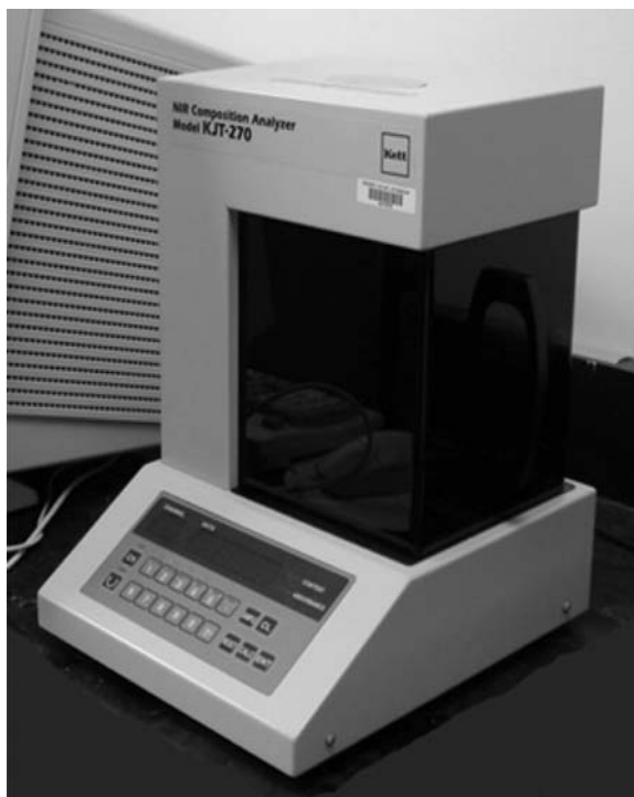
Figure 6.10 A commercial lab NIR composition meter—KJT-270 (Kett Inc., Villa Park, CA, USA).
