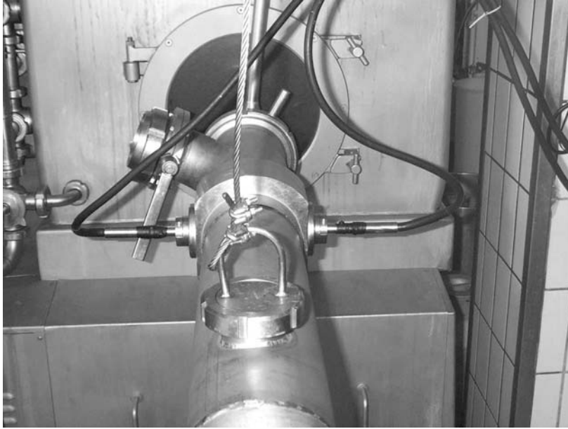
Figure 10.5 Transmission measuring device at the end of the butter-making machine. (M Sievers, 2007, personal communication)
