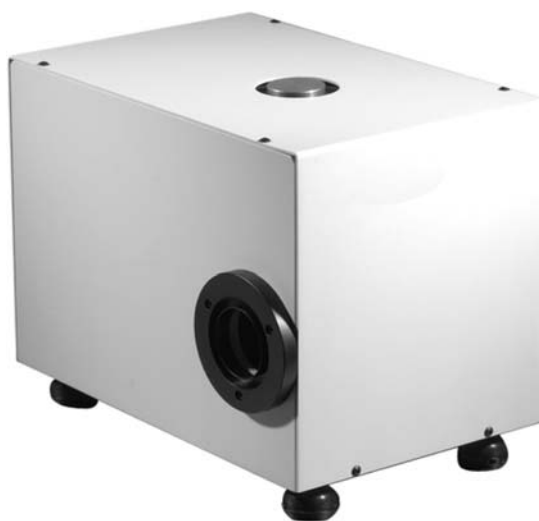
Figure 6.7 A liquid nitrogen cooled mercury cadmium telluride (MCT) detector. It has a broad spectral response close to that of deuterated triglycine sulfate (DTGS) but acquires spectral data 8 times faster than DTGS. Permission to use this photo has been granted by Newport Corporation. All rights reserved ( www.newport.com ).
