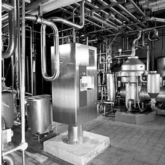
Figure 10.7 Mid-infrared measurement of fat, protein, lactose and dry matter content via a bypass. (M Sievers, 2007, personal communication)
