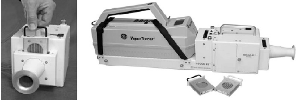
Figure 4 The miniature pre-concentrator (left) and the incorporation of the pre-concentrator with a commercial handheld IMS analyzer, known in combination as the Hound™. The metal mesh of the preconcentrator can be seen in the photo (left).
