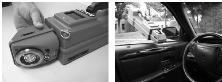
Figure 9 An ion mobility spectrometer called the Quantum Sniffer has an inlet with laser or flash-lamp to warm a surface and a vortex sampler (left frame) to pull sample into the analyzer without contact between analyzer and surface (right frame).
