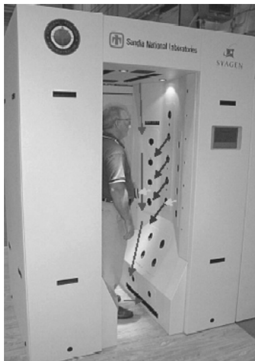
Figure 21 MS-based personnel screening portal (Reproduced from www.syagen.com/LitReq/Pres1102/portal.pdf . With permission from Sandia National Laboratories, Albuquerque, NM).
