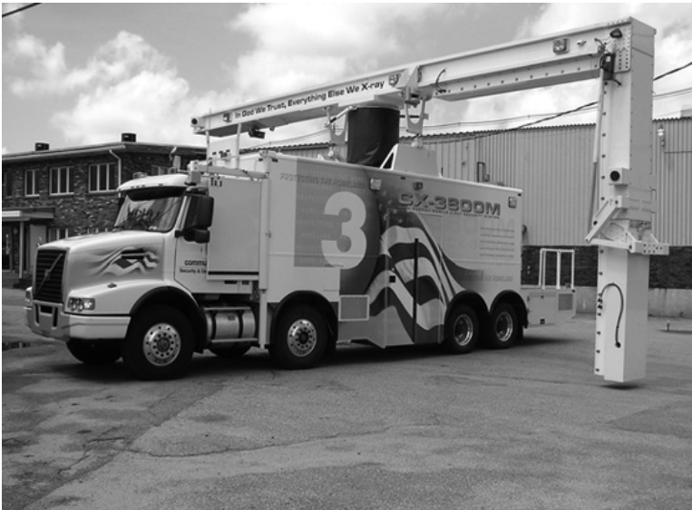
Figure 14 The CX3800M, a 3 MeV mobile cargo scanner. With the ability to penetrate over 25 cm of steel, this truck is used to X-ray other vehicles, pallets, and containers. The resulting high-definition image can be compared against the archived cargo manifest.
