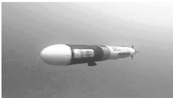
Figure 11 ICx Technologies' SeaDog underwater explosives detection sensor mounted on an autonomous underwater vehicle. Figure courtesy of ICx Technologies.
