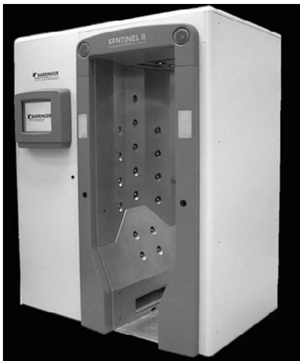
Figure 5 Portal for sampling humans for explosives. A person enters the portal and remains for some seconds while puffs of air are directed against the body and air is drawn away from the body and through a pre-concentrator.
