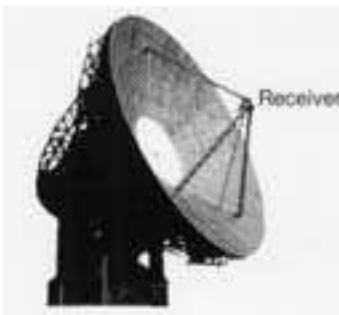
A radio antenna uses metal beams of equal length to support the receiver at its focal point.
