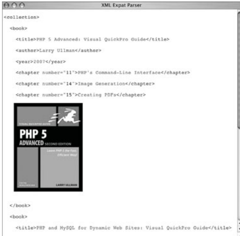
Figure 14.8 Running books3.xml through the PHP-Expat parser generates this HTML page, viewable in any browser.
