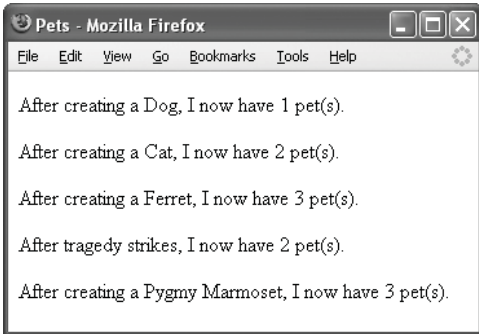
Figure 7.18 As the Pet class contains a static attribute, it can be used to count the number of objects created from derived classes.
