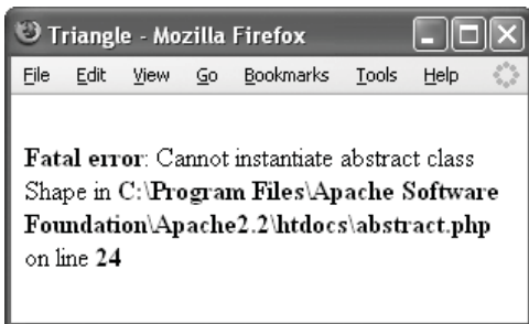
Figure 7.19 The fatal error created by trying to make an object of an abstract class.
