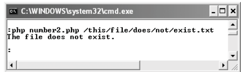
Figure 11.24 If the script cannot find the given file, an error is displayed.
