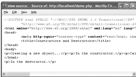
Figure 6.8 The $o object's destructor is called as the very last script event, when the script stops running. Thus, the In the destructor. messages gets sent to the browser after the closing HTML tag.
