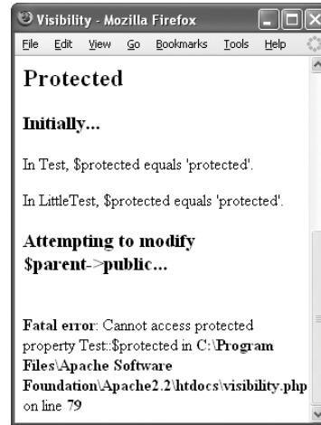
Figure 7.14 Attempting to modify the value of the protected variable using the syntax $obj->var results in a fatal error (which is bad).
