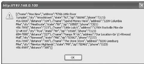
Figure 13.32 This alert reveals the data, in JSON format, received by the JavaScript from the PHP page.
