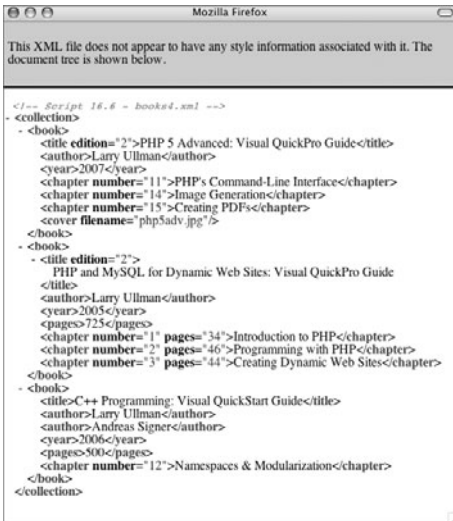
Figure 14.1 Firefox (here, on Macintosh) automatically parses an XML document to display it in a more meaningful form.
