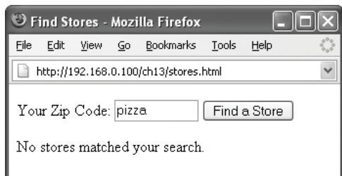
Figure 13.25 If the PHP script does not return any data, this message is displayed in the HTML page.
