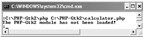
Figure 10.12 The calculator is started from the command line. If the GTK module isn't supported, it won't even try to run.
