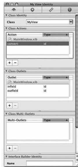
Figure 3-5 The Identity Inspector enables you to add outlets and actions to your objects. These correspond to instance variables and instance methods in your source code.
