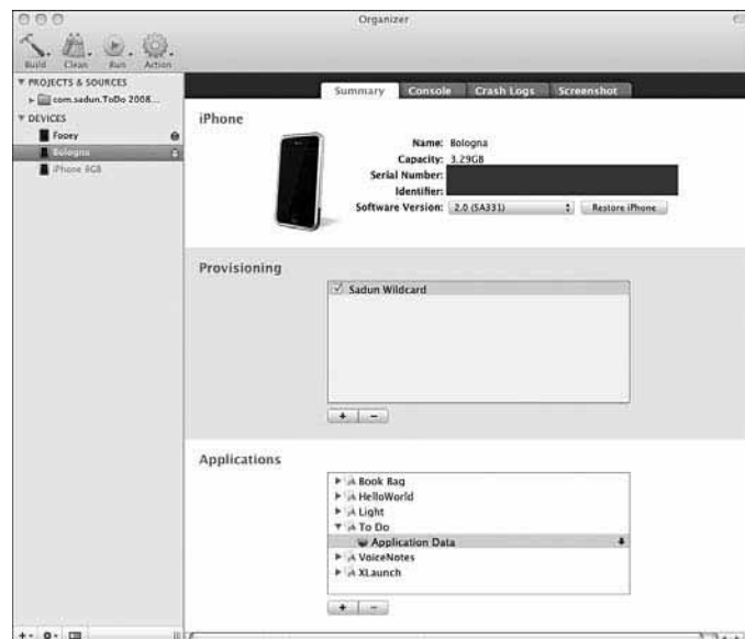
Figure 1-9 The Xcode-based iPhone Organizer window (Window, Organizer) provides a single control hub for most of your application testing needs. Here, you can load firmware, install and remove applications, read through crash logs, snap device-based screenshots, and more.
