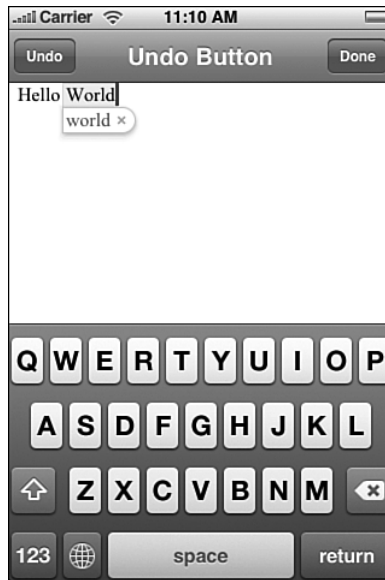
Figure 8-8 The Undo button at the top-left corner of the screen appears only after the user has changed text in the text view from the most recently stored state. Tapping Done saves any changes to the file (and hides Undo). Tapping Undo reverts the view contents to the most recently stored version.
