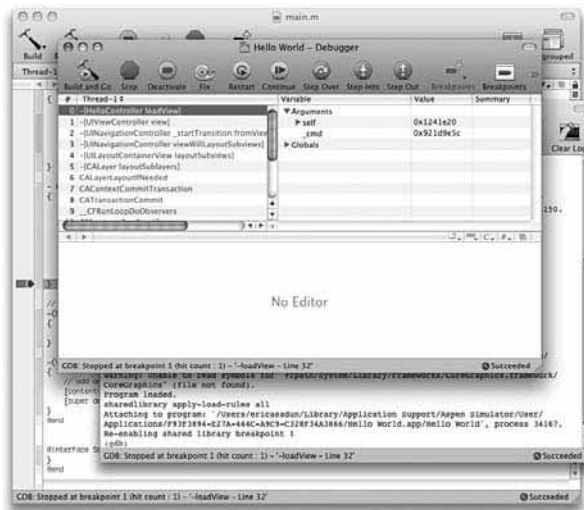
Figure 1-6 Xcode’s graphical debugger enables you to interactively inspect program state. A command-line version of gdb runs concurrently in the console window, as shown by the (gdb) prompt. A red arrow appears at the active breakpoint.
