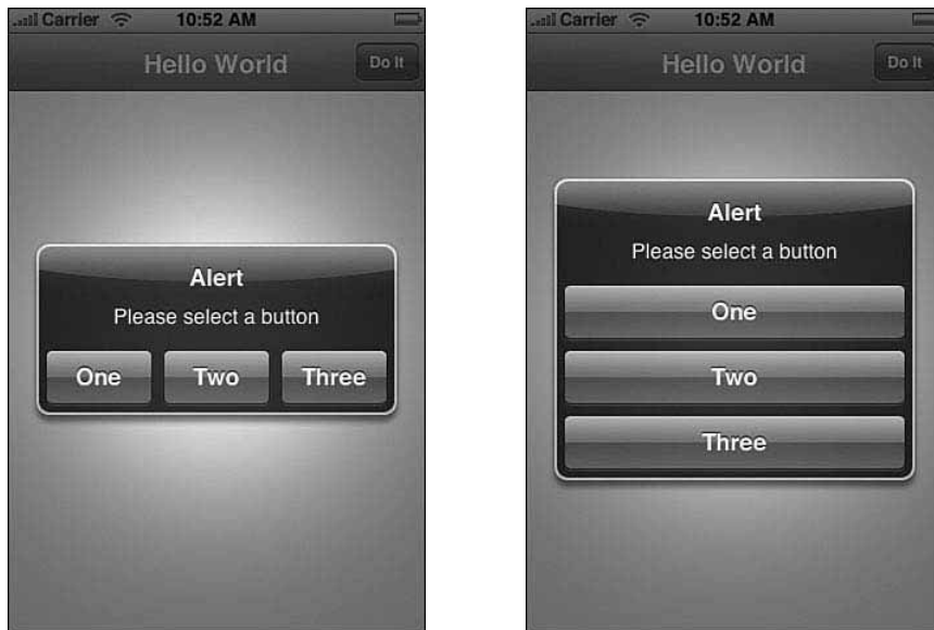
Figure 4-2 An undocumented UIKit call allows you to select whether to lay out your buttons in a row or a column.
