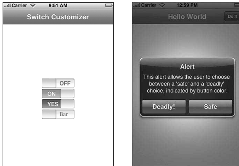
Figure 8-4 (Left) A bit of object dumpster diving allows you to expose and customize underlying UISwitch views. (Right) Color UIAlertView buttons by accessing the alert's subviews.
