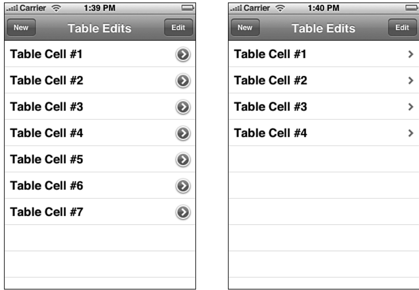
Figure 5-9 The right-pointing chevrons indicate disclosure controls, allowing you to link individual table items to another view.
