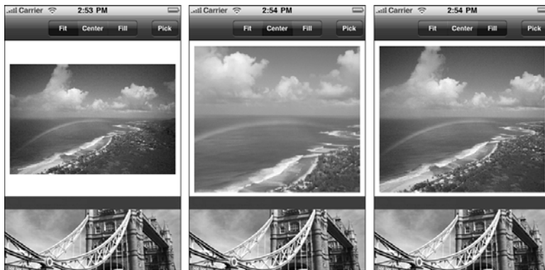
Figure 7-7 These screenshots represent three ways to create image thumbnails. Fitting (left) preserves original aspect ratios, padding the image as needed with extra space. Centering (center) uses the original image pixels, cropping from the center out. Filling (right) ensures that every available pixel is filled, cropping only those portions that fall outside the frame.
