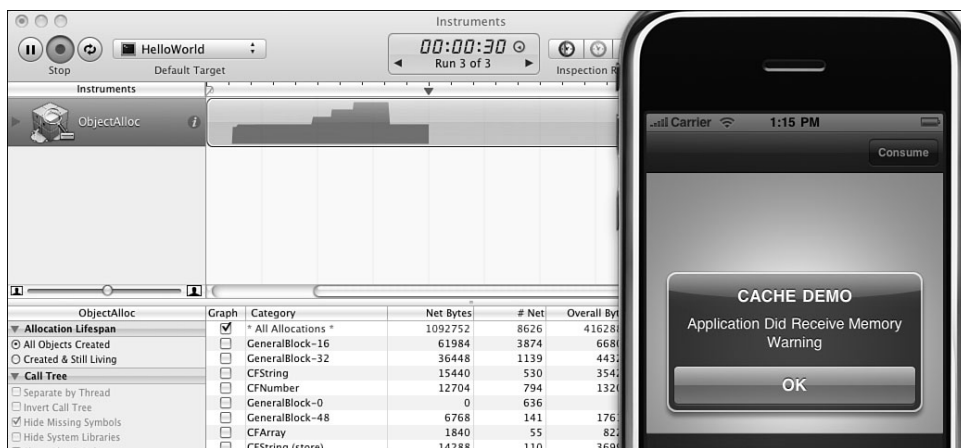
Figure 2-13 Instruments helps monitor object allocations, letting you test your release strategies during memory warnings.
