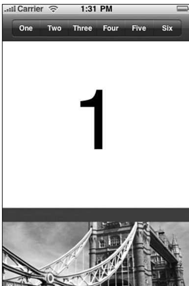
Figure 5-2 Adding a segmented control to the custom title view allows you to build a multi-item menu. Notice that no items remain highlighted even after an action takes place. (In this case, the One button was pressed.)
