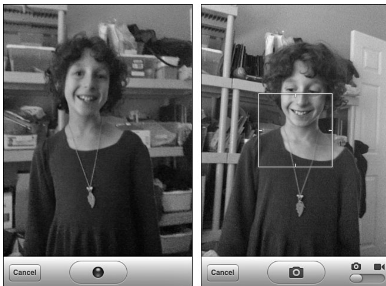
Figure 15-3 Developers may specify one or more media types for the image picker controller. The screenshot on the left demonstrates a video-only capture. The right screenshot shows a picker that supports both image and video capture.
