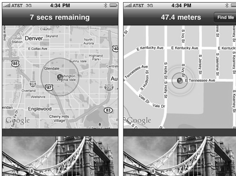
Figure 17-3 A coordinate region of a tenth of a degree latitude by a tenth of a degree longitude covers an area the size of a smallish city or large town, approximately 5 to 7 miles on a side. Shrinking that region down to 0.005 degrees on a side produces a street-level display (left). These streets lie within Denver's Garland Park/Virginia Vale neighborhood (right).
