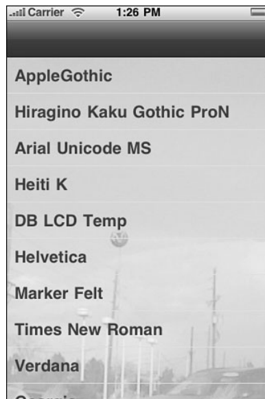
Figure 11-2 Combine a clear table background color with a backplash to create a table that scrolls over an image.
