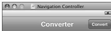
Figure 4-7 You can edit the navigation controller bar directly and add buttons to it.
