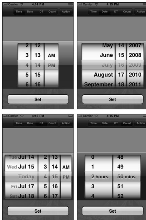
Figure 11-21 The iPhone offers four stock date picker models. Use the datePickerMode property to select the picker you want to use in your application.
