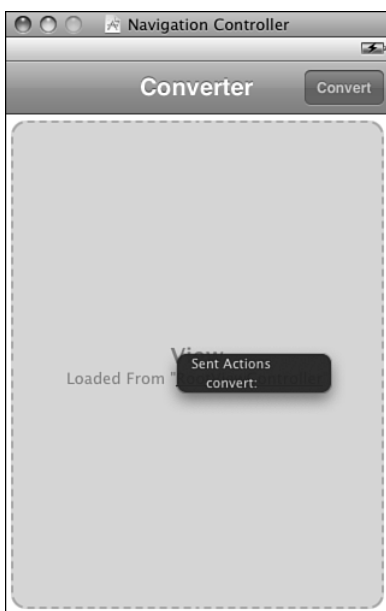
Figure 4-11 Dragging from the bar button item to the central view allows you to connect the button action to a method defined by the view's view controller.
