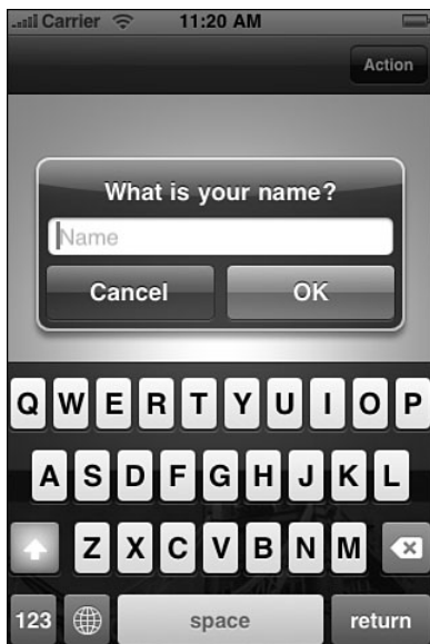
Figure 10-4 Using careful space management and omitting the title and body text, you can add several text entry fields to a UIAlertView at once. You probably want to limit your UIAlertViews to one or two text fields.
