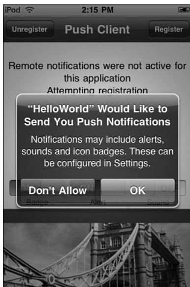
Figure 16-10 Users must explicitly grant permission for an application to receive remote notifications.
