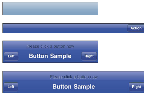
Figure 4-2 Navigation bars stretch from one side of the screen to the other. Their height is fixed at 44 pixels for portrait mode and 32 pixels for landscape on the standard iPhone. The rarely used prompt feature shown in the bottom two images zoom the bar to 74 pixels high.
