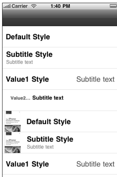
Figure 11-3 Cocoa Touch provides four standard cell types, some of which support optional images.
