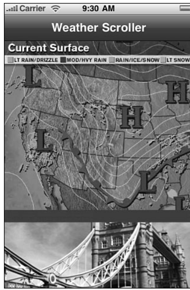
Figure 7-5 This live weather map is downloaded from a World Wide Web URL and layered onto a scroll view that allows users to scale and pan through the image.
