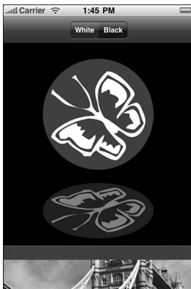
Figure 6-6 A basic Core Animation reflection uses scaling, transparency, and a slight vertical offset.
