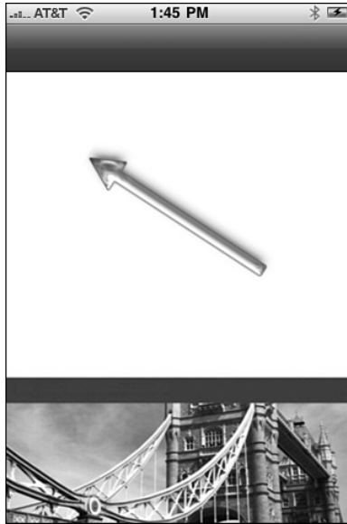
Figure 14-2 A little math recovers the “up” direction by performing an arctan function using the x and y force vectors. In this sample, the arrow always points up, no matter how the user reorients the iPhone.
