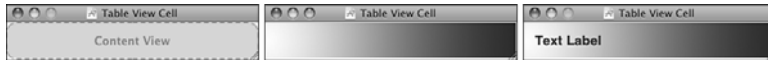
Figure 11-5 The top image shows a default cell created in Interface Builder without any content. The middle image shows that same cell after adding custom art to the cell. Adding a custom text label (bottom image) helps create a properly labeled cell like the one shown in Figure 11-4 (left).
