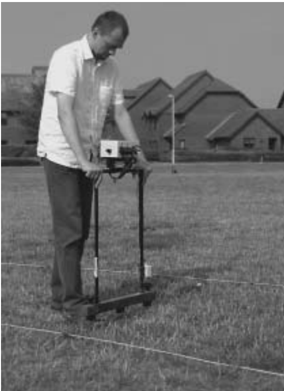
Figure 3.1 Illustrations of the Wenner configuration (top) and twin-electrode array (bottom) in use
