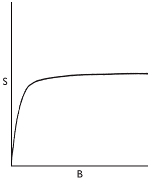
Figure 6.1 Typical Langmuir isotherm: S, concentration of substance adsorbed; B, total concentration of substance.
