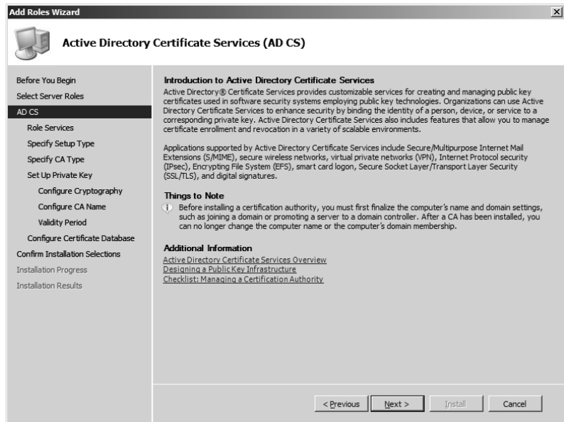
FIGURE 12.3 Active Directory Certification Services (AD CS) installation dialog box
