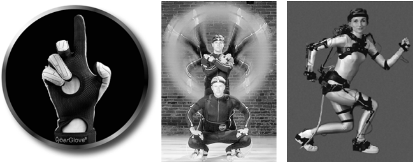
Figure 13.2. Input devices for virtual environments. (a) The CyberGlove ® for the tracking of hand movements (image courtesy of Virtual Technologies, Inc., Palo Alto, CA, USA). Finger flexion is monitored with fiber optics and a position sensor can be attached to track the position and orientation of the hand in space. (b) The STAR*TRAK ® system captures position and motion of the whole body with an electromagnetic system (image courtesy of Polhemus Inc., Colchester, VT, USA). (c) The Gypsy ™ 2.5 Motion Capture System analyzes whole body motion on the basis of potentiometers (image courtesy of Analogus ™ Corp., Fremont, CA, USA).
