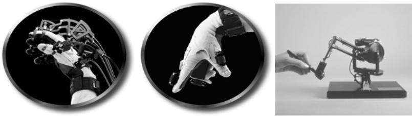
Figure 13.5. Systems for haptic feedback. (a) CyberTouch TM provides vibrotactile stimulators on each finger and the palm of the hand (image courtesy of Virtual Technologies, Inc., Palo Alto, CA). (b) CyberGrasp TM features resistive force feedback for the hand from dc motors (image courtesy of Virtual Technologies, Inc., Palo Alto, CA). (c) The Phantom Premium 3D systems are high-fidelity desktop devices that can generate high forces (image courtesy of SensAble Technologies, Inc., Cambridge MA).
