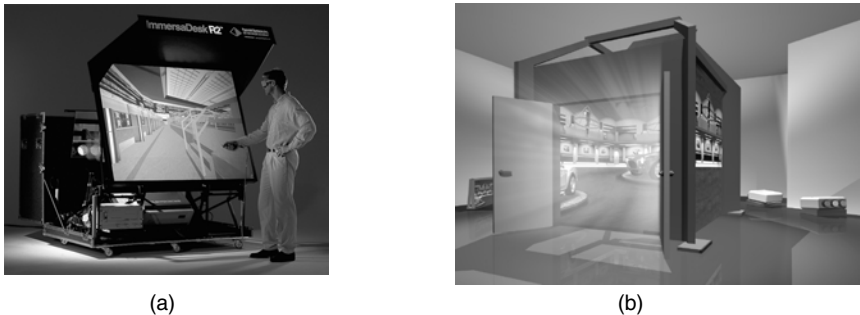
Figure 13.4. The ImmersaDesk R2 (a) and the CAVE™ (b) use shutter glasses and large rear projectors to immerse one or more users into a virtual environment. The display is adjusted to the tracking of head movements and the user can interact with the environment, for example with 3D input devices (images courtesy of Fakespace Systems, Mountain View, CA).
