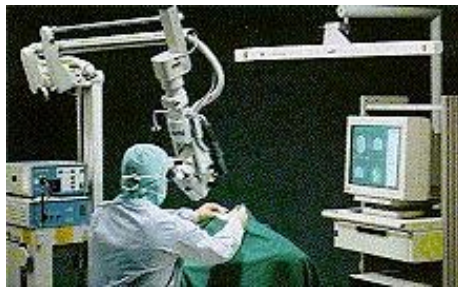
Figure 12.8. The multicoordinate manipulator system (MKM) from Zeiss. The carrier of the microscope can be controlled by foot, hand, mouth or voice. Information on target areas identified during surgery planning can be superimposed onto other images in the microscope and on the screen.
