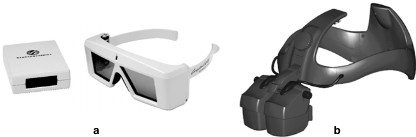
Figure 13.3. Eyewear for visual display of virtual environments. The CrystalEyes ® in (a) are shutter glasses that alternately block and pass light for each eye and are used with stereoscopic displays. Synchronization of display and glasses is achieved with infrared signals from the emitter shown to the left (image courtesy of StereoGraphics Corp., San Rafael, CA). The ProView ™ XL50 in (b) is a head-mounted display that can deliver stereographic full color images at high resolution (image courtesy of Kaiser Electro-Optics Inc., Carlsbad, CA).
