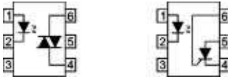
Fig. 2.31. An optically-coupled triac and thyristor
