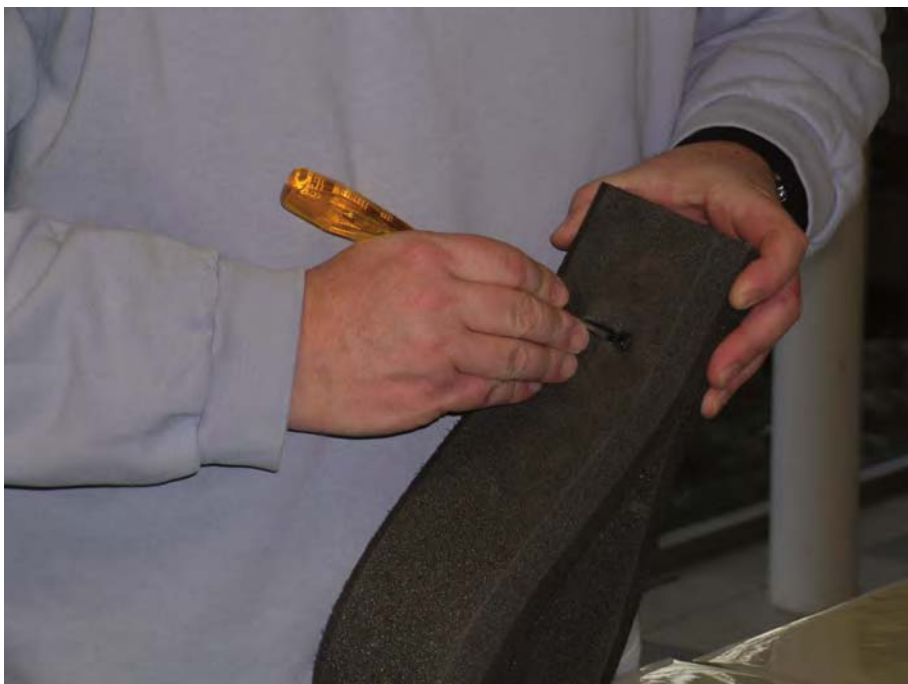
Figure 23.51 The mechanism is then pushed into the foam to hide it from view. The mount can then be pushed into the base; this can be bonded if necessary.
