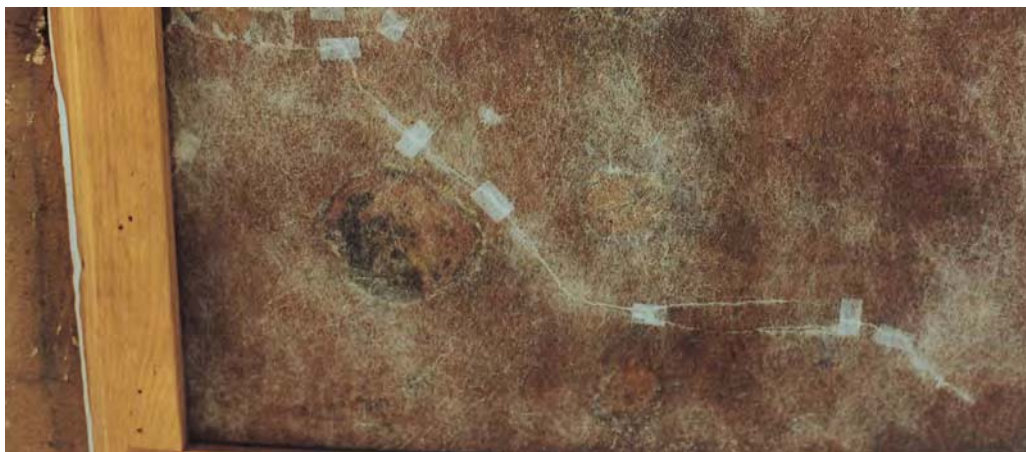
Figure 23.77 Patches of Japanese tissue paper along the join to hold it in place as the lining is applied. The Reemay has been applied over them.
