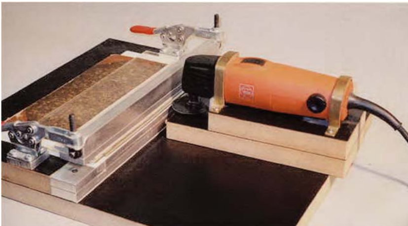
Figure 21.11 Minter's mounted FEIN MultiMaster with oscillating saw blade for board slotting is advanced by hand to create a slot in the edge of the binderboard which is clamped in the jig.
