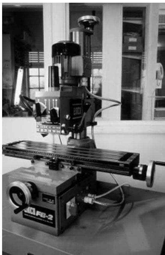
Figure 21.8 The milling machine Emco FB-2, used for the board slotting technique by the Bodleian Library.
