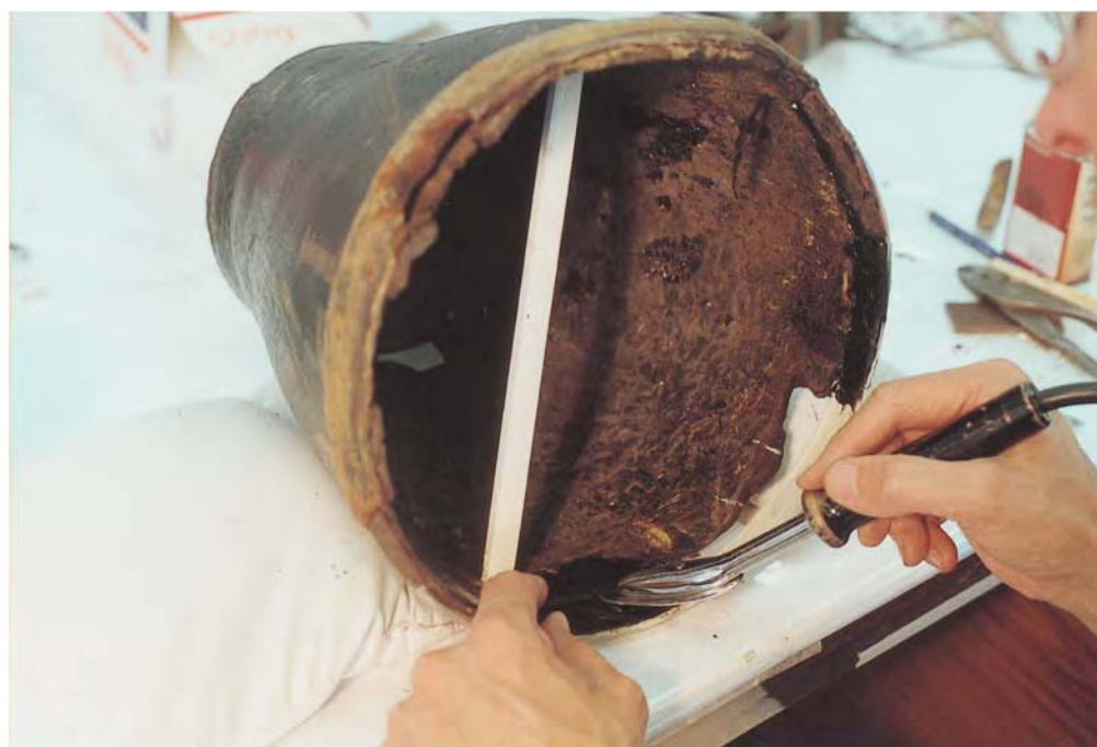
Figure 23.10 Building up the missing section with solid Beva 371 and a heated spatula.
