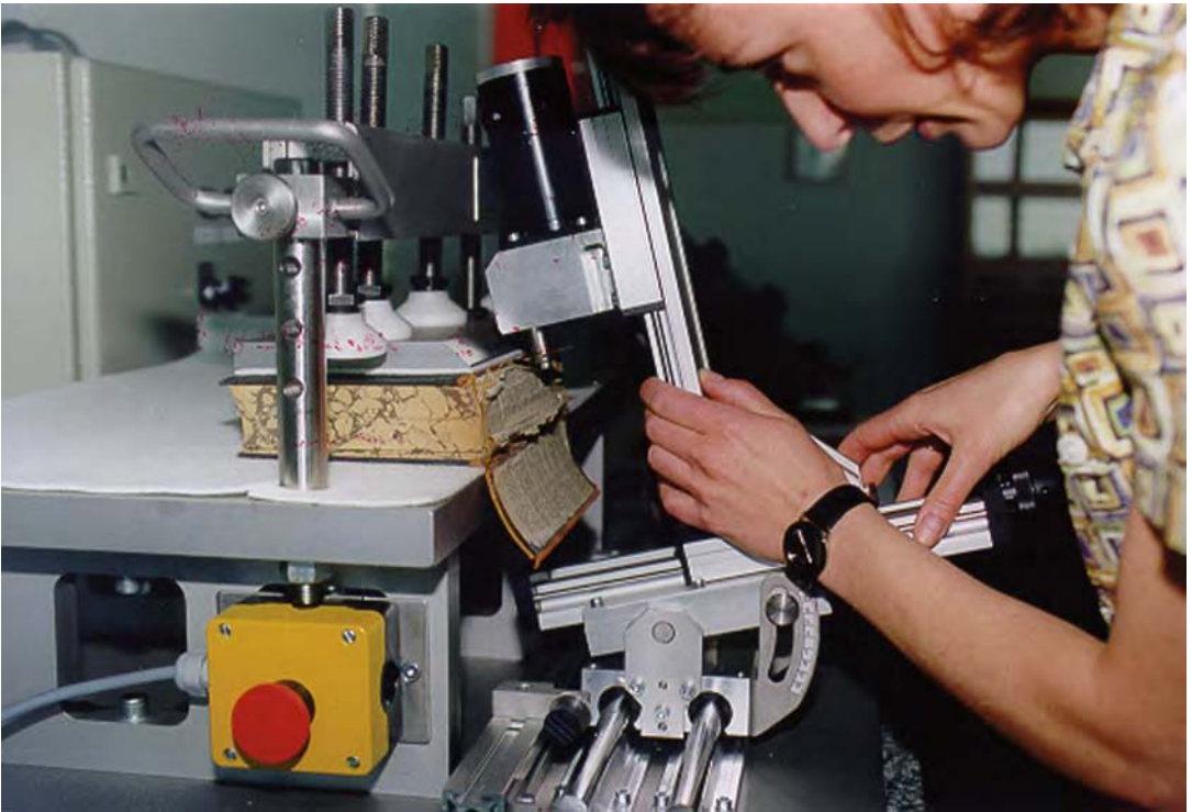
Figure 21.9 The board slotting machine developed by Becker Preservotec in cooperation with the Academy of Art and Design, Stuttgart.
