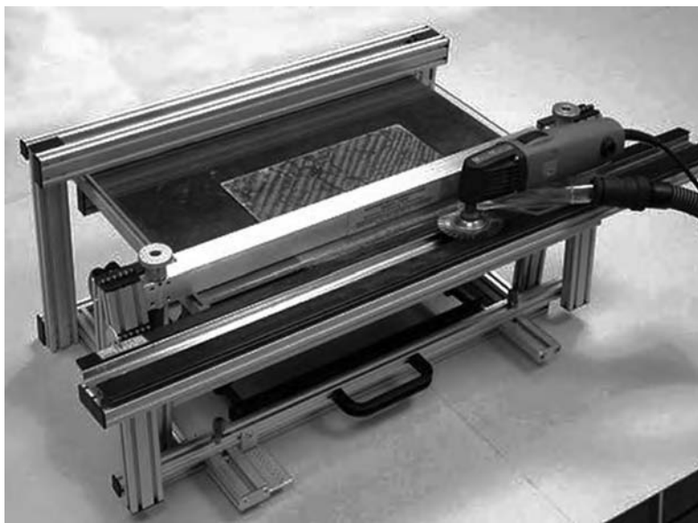
Figure 21.12 Mayer's mounted FEIN MultiMaster for board slotting from the University Library of Graz, Austria.
