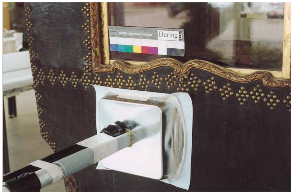
Figure 23.22 Low pressure suction box.
